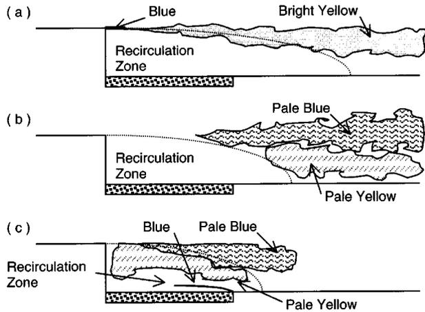
**Fig. 2** Flame stabilization and suppression regimes. (a) Rim-attached wrinkled laminar flame at low air velocities, (b) transition flame, and (c) wake-stabilized turbulent flame at high air velocities.
