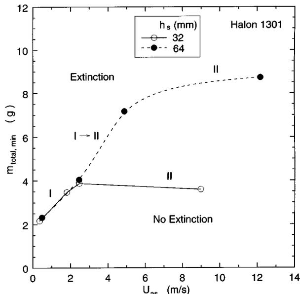
Fig. 7 The minimum total agent mass at suppression as a function of mean air velocity at the step with corresponding flame stabilization and suppression regimes.
