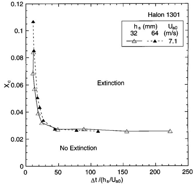
**Fig. 5 The critical agent mole fraction at suppression as a function of non-dimensional agent injection period for a high air velocity**
