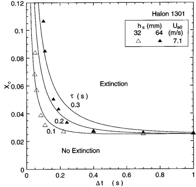
**Fig. 4 The critical agent mole fraction at suppression as a function of agent injection period for a high air velocity with theoretical fitting curves for different characteristic mixing times.**
