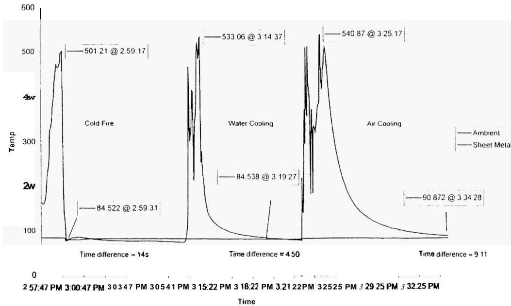
Figure 2. Cold fire cooling on sheet metal
