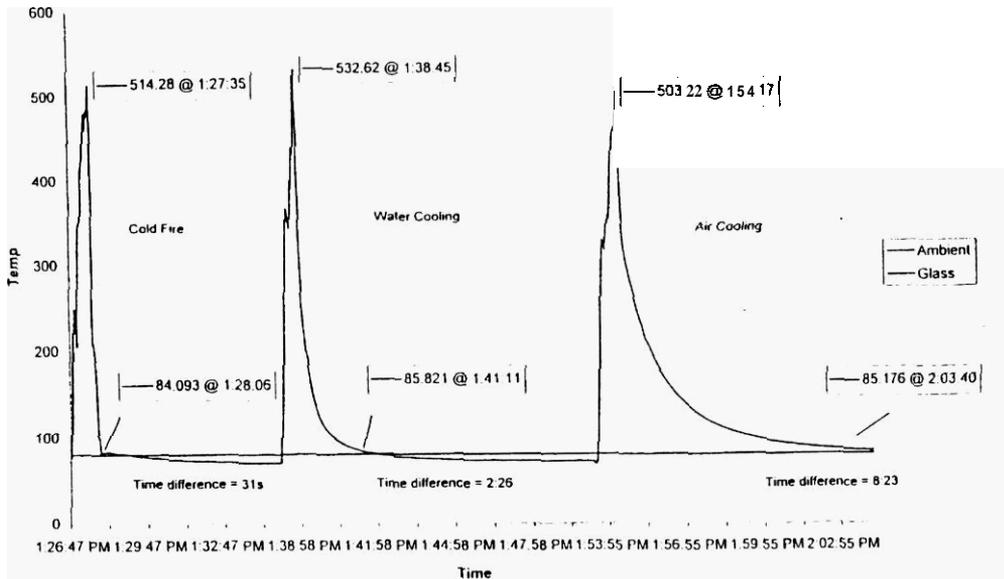
Figure 3. Cold fire cooling on glass.
