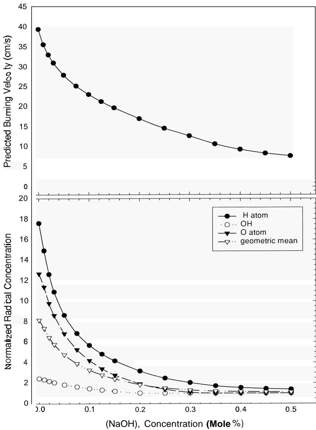
Figure 1. Predicted flame speed (top) and radical concentration overshoot (bottom) for methane/air mixtures inhibited by  $\text{Na}_2\text{O}_2\text{H}_2$ .
