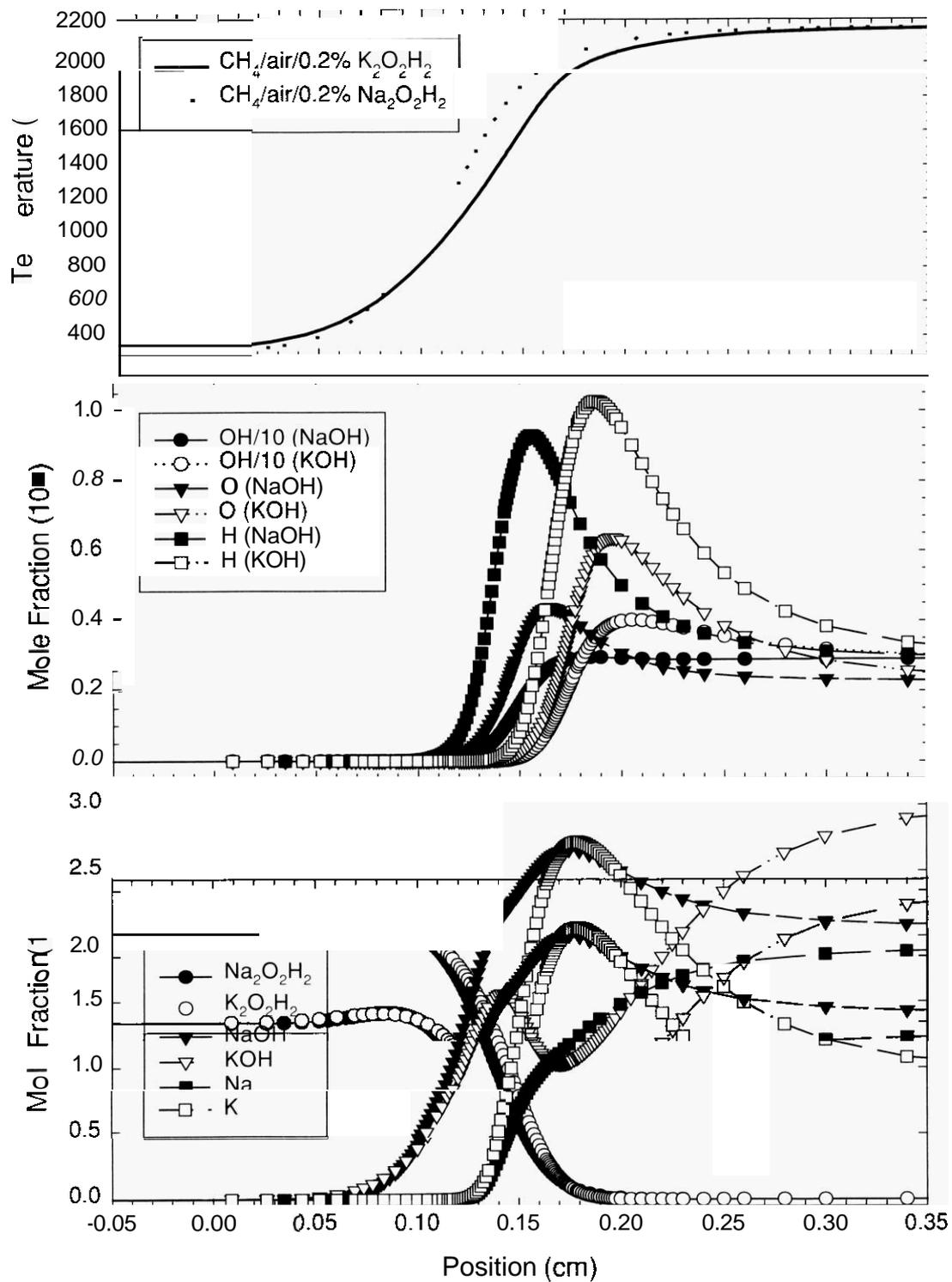
Figure 2. Predicted profiles of temperature (top), key flame radicals (middle), and alkali metal species (bottom) in methane/air flames inhibited by sodium and potassium hydroxide.
