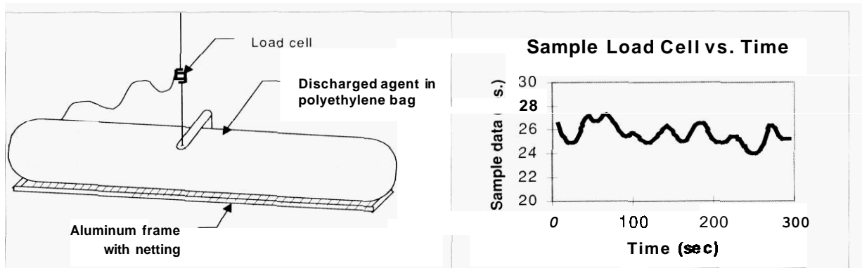
Figure 2. Load cell weighing, sketch, and data.
