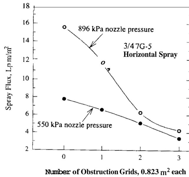
**Figure 4** The effect of obstruction grids on spray flux density of 3/4 7G-5 nozzle in spray plenum, at different nozzle pressures.
