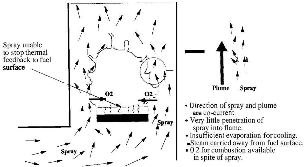
Figure 5 (a). Water mist supplied from below the flame.
