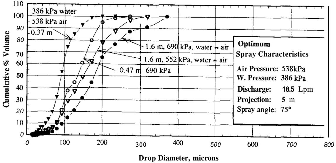
Figure 2 Dropsize distribution curves for 1/2J SU89 air-atomizing nozzle.
