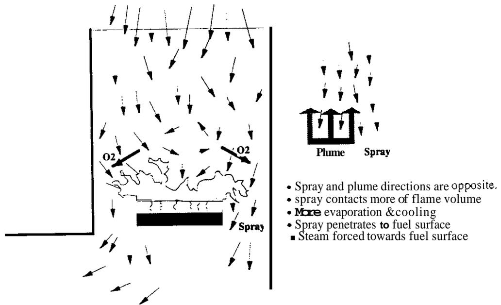
Figure 5 (b). Water mist supplied with momentum from above the flame.
