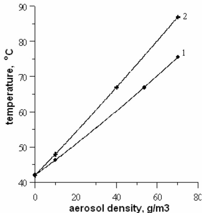
**Figure 1. The dependence of mean temperature in enclosure (V=0.11 m<sup>3</sup>) at application of aerosols for extinguishing of ethanol pool fire.**
