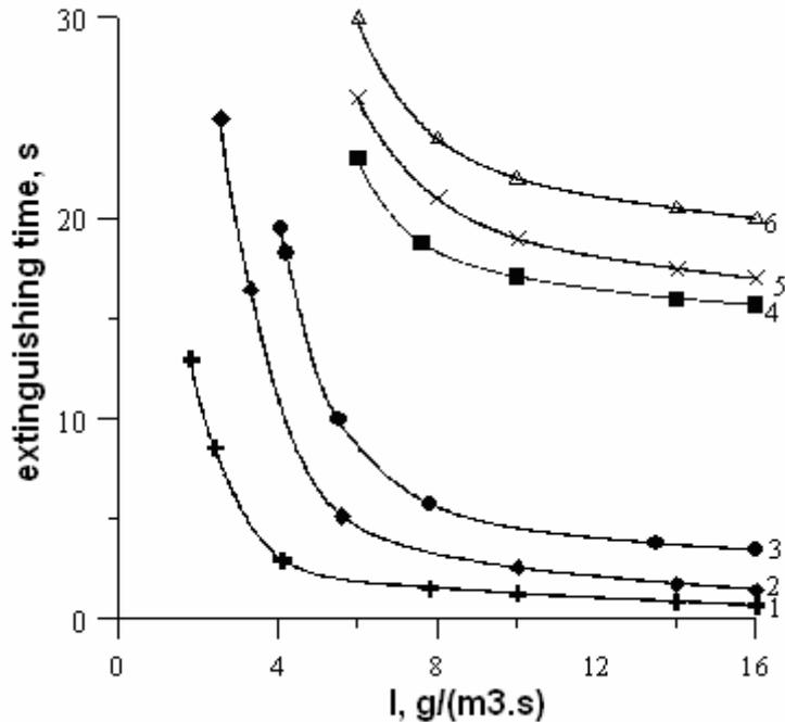
**Figure 5. Dependence of extinguishing time for gasoline on intensity of aerosol supply into protected volume: 1 – simultaneous supply of the aerosol into the enclosure and into the cabinet; 2,3 – direct supply of the aerosol into the cabinet; 4-6 – total flooding by condensed aerosol in the enclosure for various square of model fire  $S$  (1,2,6 -  $S = 0.006 \text{ dm}^2$ ; 5 -  $S = 0.03 \text{ dm}^2$ ; 3,4 -  $S = 0.49 \text{ dm}^2$ )**
