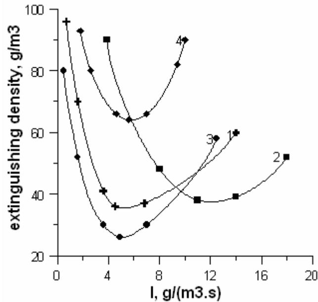
**Figure 3. Dependence of extinguishing density of the aerosol on intensity of its supply into protected volume. Aerosol forming compound – SBK-2. Combustible – PMMA.**
