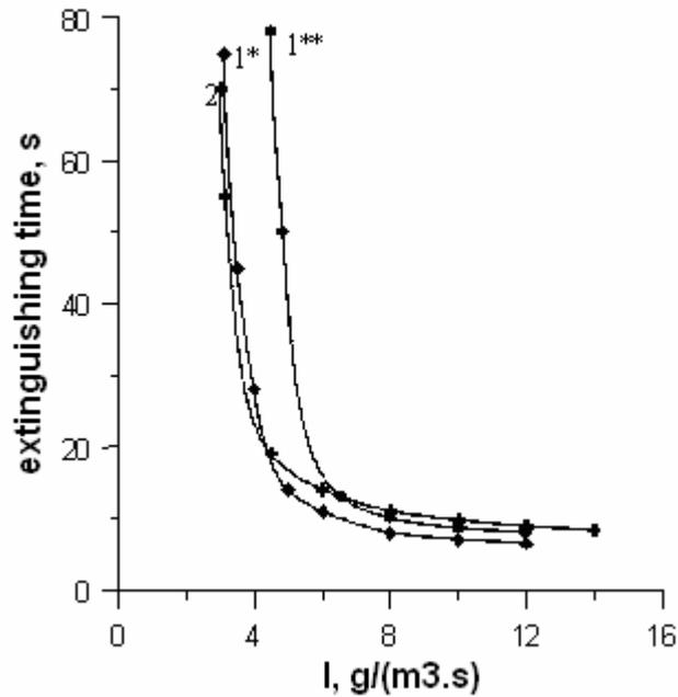
**Figure 4. Dependence of extinguishing time for PMMA on intensity of aerosol supply into protected volume. Aerosol forming compounds: 1\* - STK-2MD ( $T_c \sim 950 \text{ }^\circ\text{C}$ ;  $T_c$  – temperature of combustion), 2 – STK-5-1 ( $T_c \sim 1100 \text{ }^\circ\text{C}$ ), 1\*\* - SBK-2 ( $T_c \sim 1250 \text{ }^\circ\text{C}$ )**
