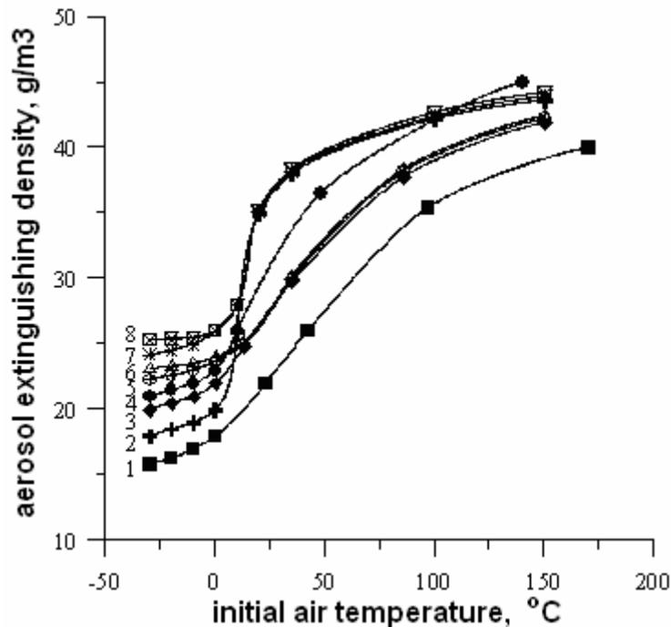
**Figure 2. The dependence of aerosol extinguishing density for various combustibles (1-PVC; 2,7,8- gasoline A-76; 3,5,6-rubber; 4-PMMA) on initial air temperature in the enclosure and preburning time (1-4 - 10 s; 5,7 - 30 s; 6,8 s - 60 s).**
