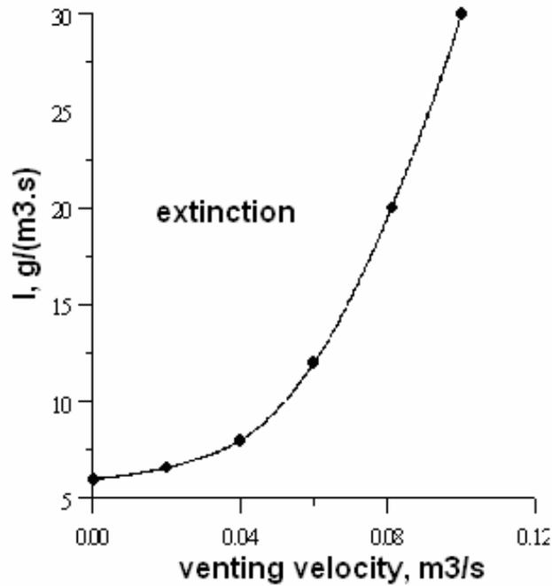
**Figure 7. Dependence of intensity of aerosol supply directly into the cabinet on venting velocity**
