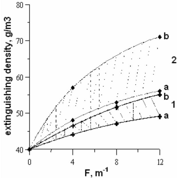
**Figure 6. An influence of surface of electrical units and their arrangement on efficiency of fire extinguishing in cabinets with electrical equipment. Surface: a – smooth, b – rough. Arrangement: 1 - separate elements or group(s) of units which not allow existence of flows in channels; 2 - structures with channels. Aerosol forming compound: STK-2MD**
