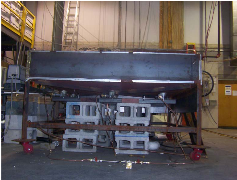
Figure 7 - Photograph Showing Below Deck Heating Burners
