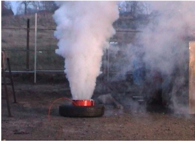
Figure 2. Discharge of a single rapid discharge extinguisher unit
