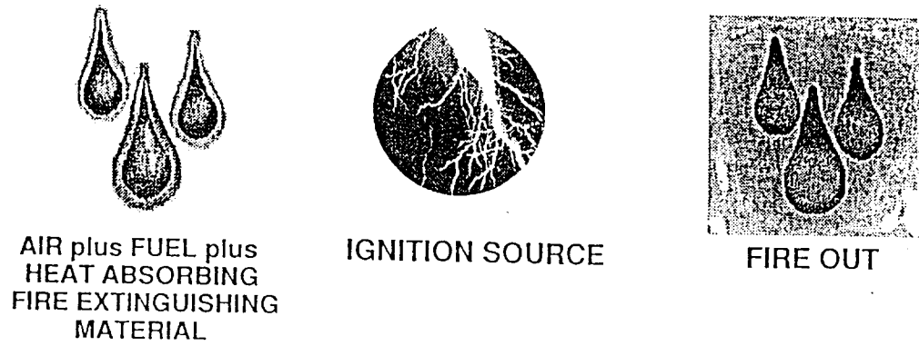
Figure 5. Ignition of a fuel-air mixture containing a heat-absorbing agent.
