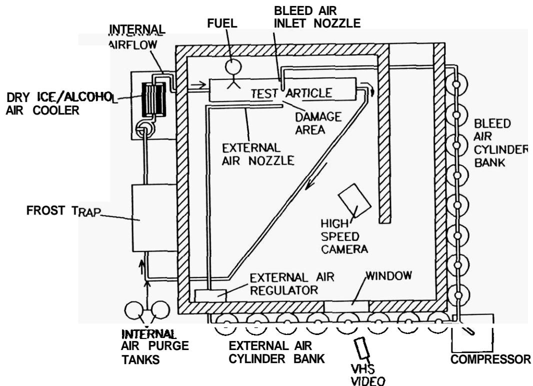
**FIGURE 3: 12 FT<sup>3</sup> DRY BAY TEST VESSEL CONFIGURATION**
