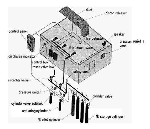
Figure 3. Typical Nitrogen Total-Flood Fire Suppression System Layout.
