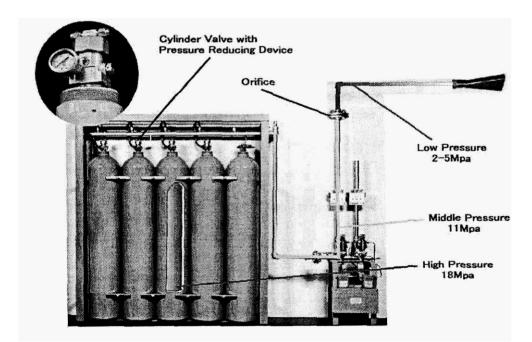
Figure 2. Typical Components of a Nitrogen Gas Total-Flood Fire Suppression System.
