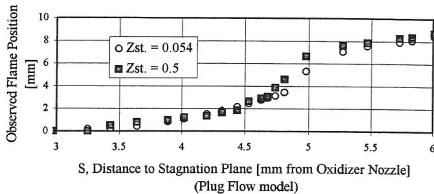
Figure 3. Variation of Observed Flame Position with the parameter S.
