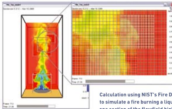
Calculation using NIST's Fire Dynamics Simulator (FDS) software to simulate a fire burning a liquid hydrocarbon fuel. A blow-up of one section of the flowfield highlights computational techniques being developed to enable more accurate calculations.
