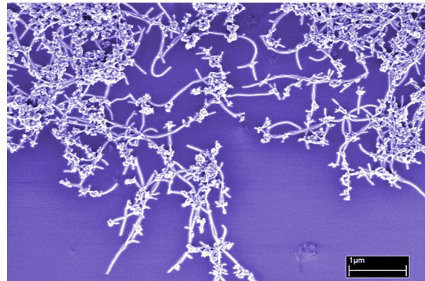
A new NIST measurement method rapidly determines the quality of a carbon nanotube sample.
