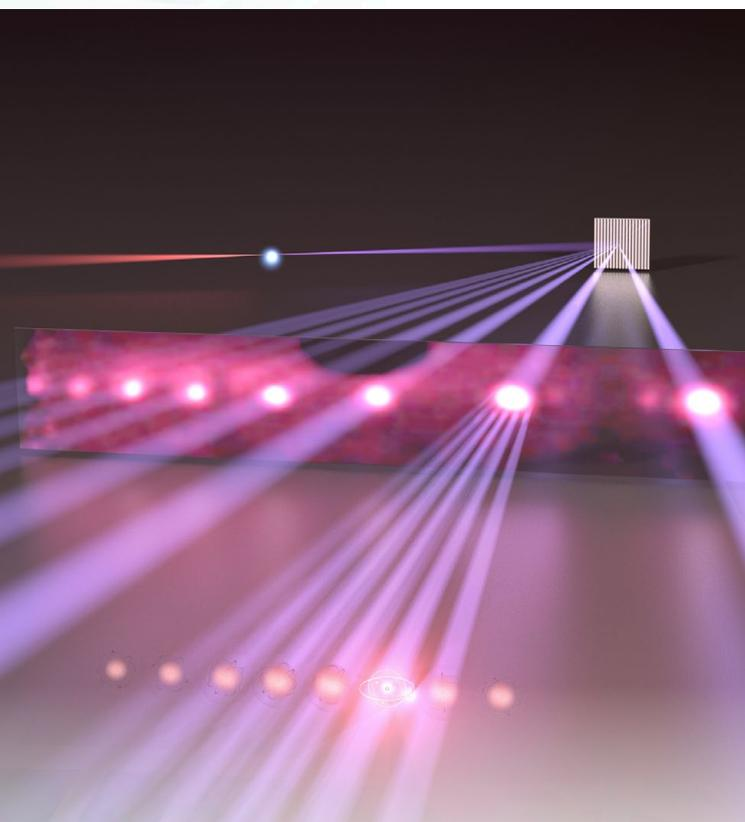
**Artist's conception of the first "frequency comb" in the extreme ultraviolet band of the spectrum, which contains high-energy light less than 100 nanometers (nm) in wavelength, created by physicists at JILA. Laser-generated frequency combs are the most accurate method available for precisely measuring frequencies, or colors, of light** (Credit: Baxley/JILA)
