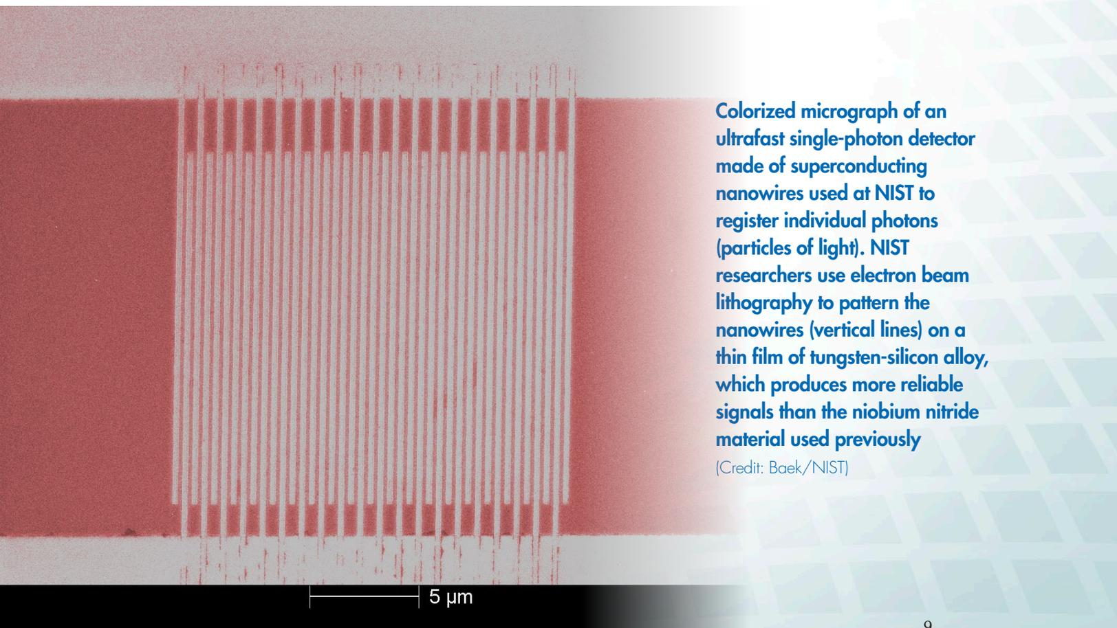
**Colorized micrograph of an ultrafast single-photon detector made of superconducting nanowires used at NIST to register individual photons (particles of light). NIST researchers use electron beam lithography to pattern the nanowires (vertical lines) on a thin film of tungsten-silicon alloy, which produces more reliable signals than the niobium nitride material used previously**
