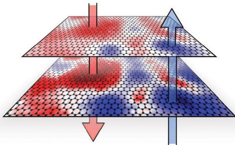
**NIST measurements show that interactions of the graphene layers with the insulating substrate material causes electrons (red, down arrow) and electron holes (blue, up arrow) to collect in "puddles". The differing charge densities creates the random pattern of alternating dipoles and electron band gaps that vary across the layers.** (Credit: NIST)
