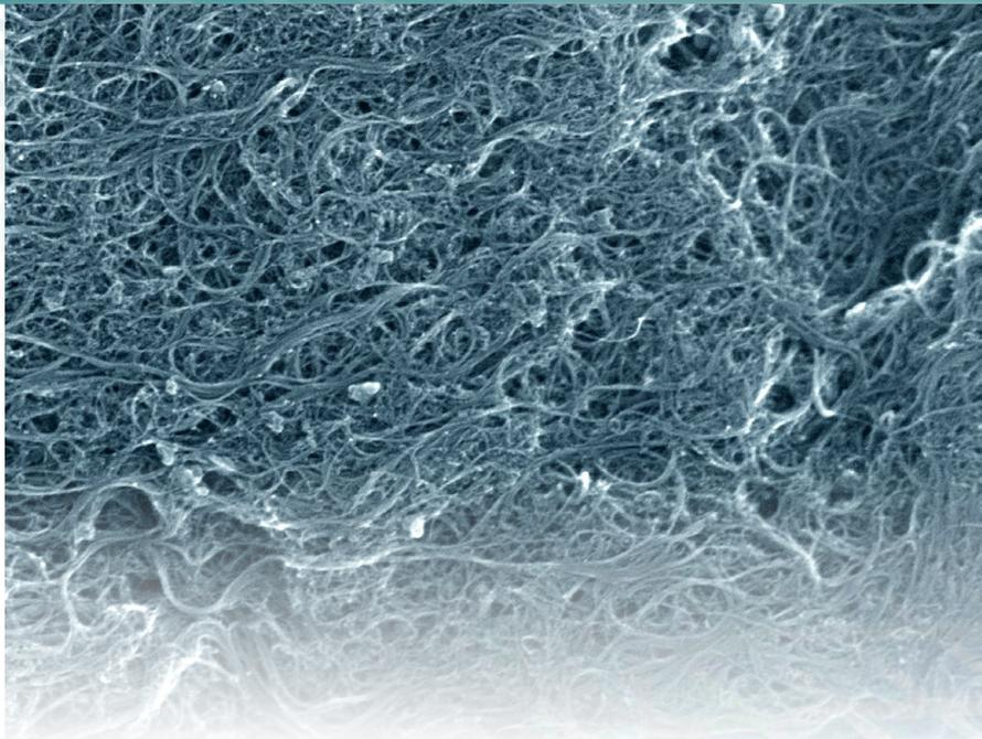
**NIST has issued the world's first reference material for single-wall carbon nanotube soot, which offers companies and researchers a highly reliable source of uniform and well-characterized carbon nanotube soot for material comparisons, as well as chemical and toxicity analysis** (Credit: Vladar/NIST)
