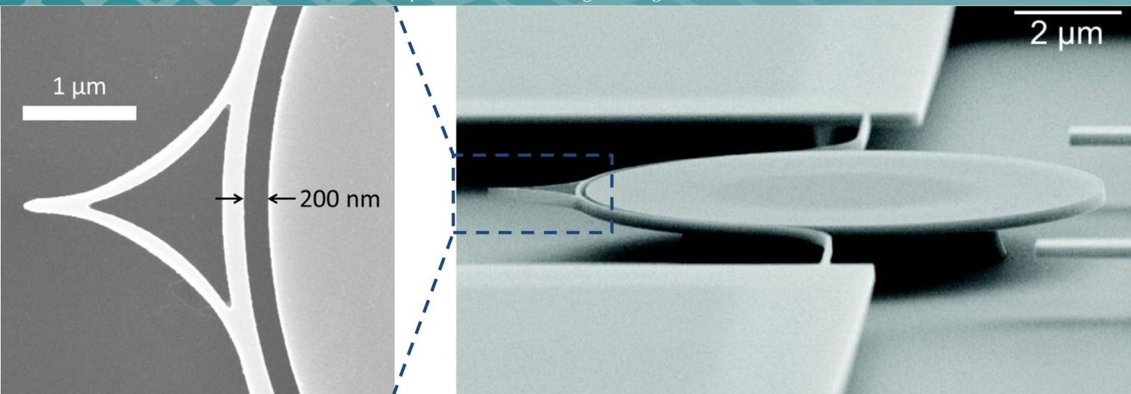
**CNST researchers developed a nanomechanical cantilever probe with a high-sensitivity nanophotonic interferometer on a single silicon chip. Replacing the traditional bulky laser detection system with this integrated device allows cantilevers that are orders of magnitude smaller than those used in conventional atomic force microscopy to be built. This innovation creates opportunities for rapid, compact, and low-cost nanoscale metrology for a wide range of applications.** (Credit: NIST)
