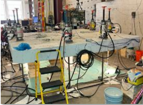
Laboratory slab-column connection tests
