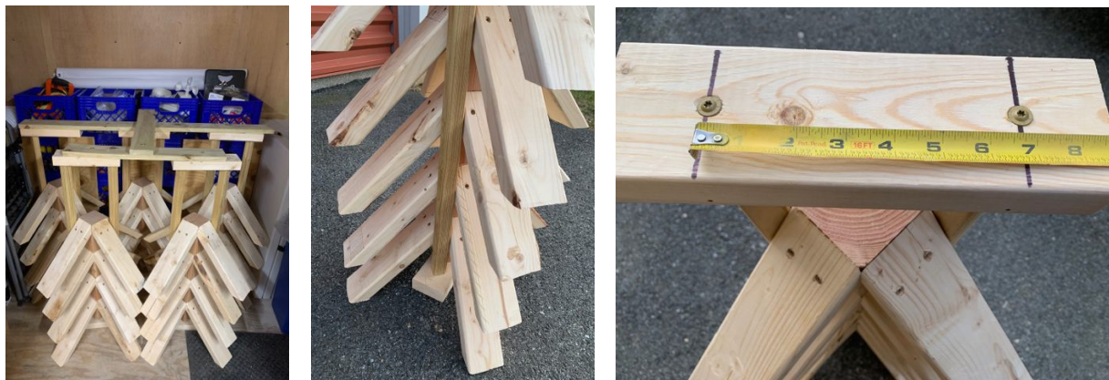
Figure 5: LEFT) For multiple lane transport, stands stack in sets without buckets in fabricated carry caddies. CENTER) The carry caddy is made of 5x5x30cm (2x4x12in) top and bottom pieces, with 5x5x90cm (2x2x36in) balusters placed vertically between where the stand legs meet. RIGHT) The balusters are spaced about 18cm (7in) apart so the balusters nest in between the legs against the center posts. Unscrew the top to insert the stands and replace for carrying.
