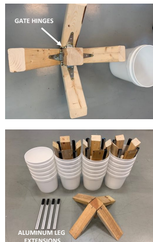
Figure 3: LEFT) These small omni bucket stands can be stacked, stowed, and ready to lay out in minutes with their associated Launch/Land Platform and a measuring tape. CENTER LEFT) For multiple lane transport, the stands can be stacked in fabricated caddies with the buckets stacked separately. CENTER RIGHT) The stands can have gate hinges at the joints to stow even smaller. RIGHT) All four hinged stands and buckets fit into two golf bags for transport. The Launch/Land Platform needs to be cut down into 12in strips with duct-taped seams acting as “accordion hinges” to fit in the golf bag along with all the buckets. The sensor panels can be cut down and taped similarly. So an entire Open Test Lane fits into two golf bags.
