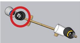
Attach bucket with a single center screw before applying this sticker to the inner base. After installation, rotate so sticker is upright.
