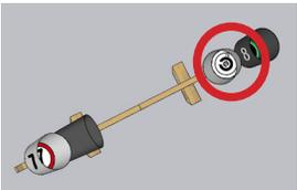
Attach bucket with a single center screw before applying this sticker to the inner base. After installation, rotate so sticker is upright.
