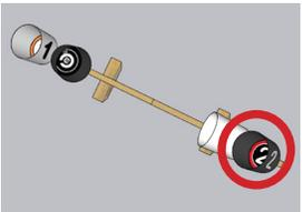
Attach bucket with a single center screw before applying this sticker to the inner base. After installation, rotate so sticker is upright.
