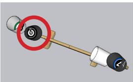
Attach bucket with a single center screw before applying this sticker to the inner base. After installation, rotate so sticker is upright.
