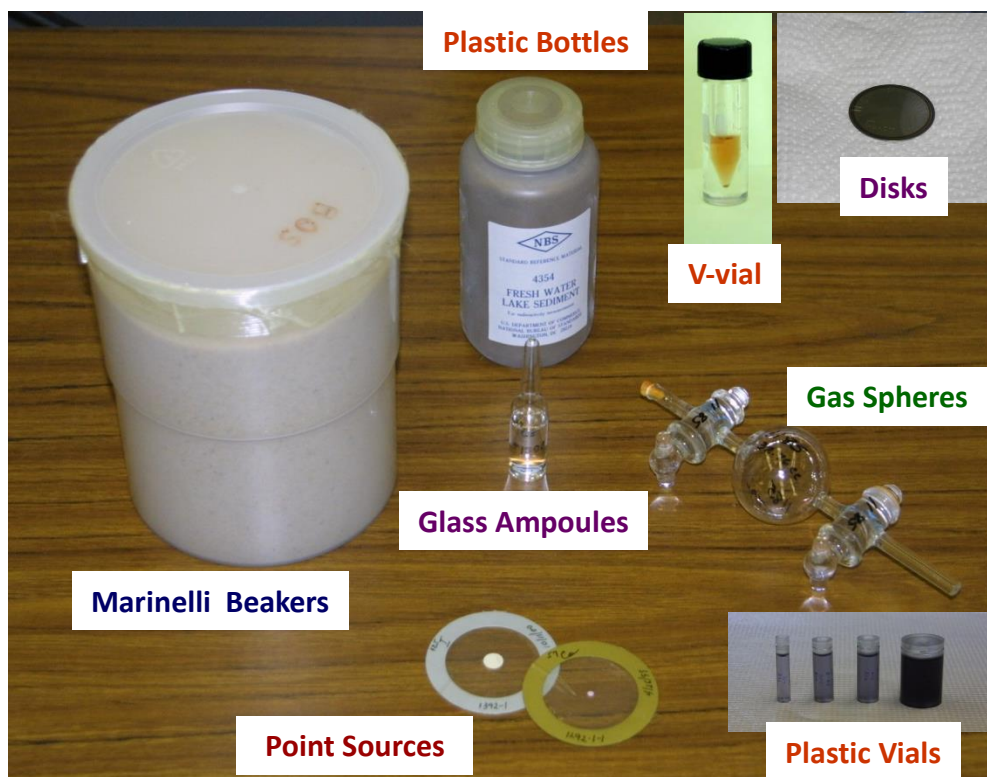
Figure 1: Picture showing the different source types measured in the HPGe detectors
