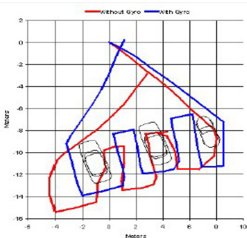
Figure 3. Manufacturer's demo of gyro-stabilized dead reckoning module improvement (from [13]).
