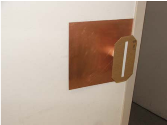
Figure 6. RFID tag and metallic backing placed on hallway wall.
