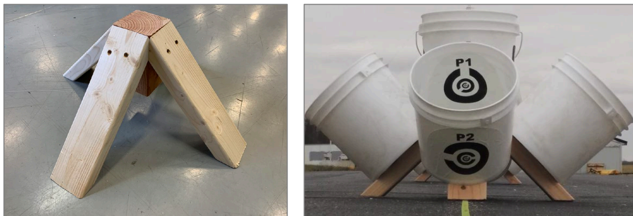
Figure 9: All four angled 5x10x30in (2x4x12in) legs with tapered ends attach aligned to the top of the center post using two 7.5cm (3in) long washer head screws. Start the screws at a 45deg angle into the legs while on the ground before attempting to affix to the center post. The top bucket mounts to the center post end grain using the same two 7.5cm (3in) long washer head screws. These need to be long to carry the weight of the entire assembled stand in the end grain. Leave the handle on the top center bucket only as a carry handle for the assembled bucket stand. The ANGLED BUCKETS SHOULD BE TOUCHING THE TOP BUCKET to support it when stacked. NOTE: Drill small drain holes in the bottom of the buckets if they are to remain outside. The parts required to construct a lane include the following. See the online USAGE GUIDE for fabrication details and pointers:
