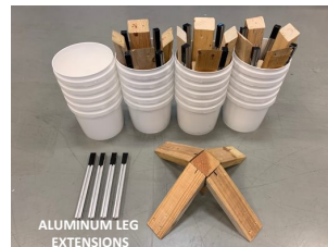
Figure 3: LEFT) These small omni bucket stands can be stacked, stowed, and ready to lay out in minutes with their associated Launch/Land Platform and a measuring tape. CENTER LEFT) For multiple lane transport, the stands can be stacked in fabricated caddies with the buckets stacked separately. CENTER RIGHT) The stands can have gate hinges at the joints to stow even smaller. RIGHT) All four hinged stands and buckets fit into two golf bags for transport. The Launch/Land Platform needs to be cut down into 12in strips with duct-taped seams acting as “accordion hinges” to fit in the golf bag along with all the buckets. The sensor panels can be cut down and taped similarly. So an entire Open Test Lane fits into two golf bags.
