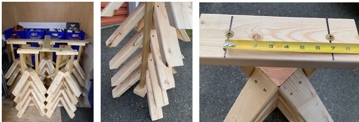
Figure 5: LEFT) For multiple lane transport, stands stack in sets without buckets in fabricated carry caddies. CENTER) The carry caddy is made of 5x5x30cm (2x4x12in) top and bottom pieces, with 5x5x90cm (2x2x36in) balusters placed vertically between where the stand legs meet. RIGHT) The balusters are spaced about 18cm (7in) apart so the balusters nest in between the legs against the center posts. Unscrew the top to insert the stands and replace for carrying.
