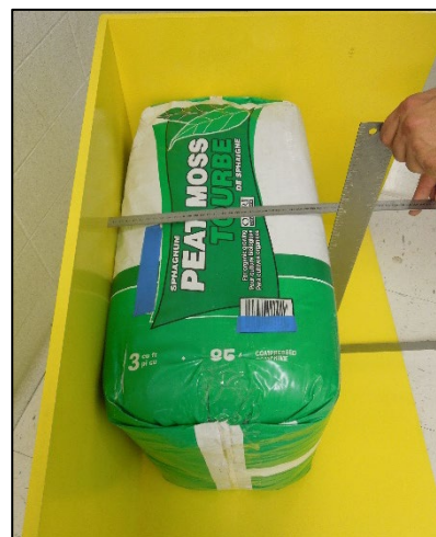
Figure 3-6. Width Measurement. The frame is rotated on its end to vertical so that the carpenter square does not compress the product.
