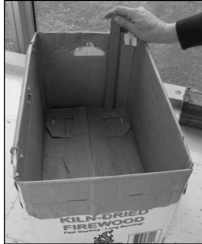
Figure 3-8. Measuring the Internal Height of the Box.
