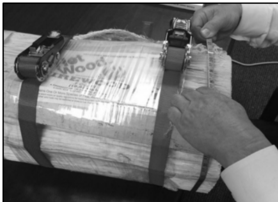
Figure 3-13a. Strapping the Ends of a Bundle.
