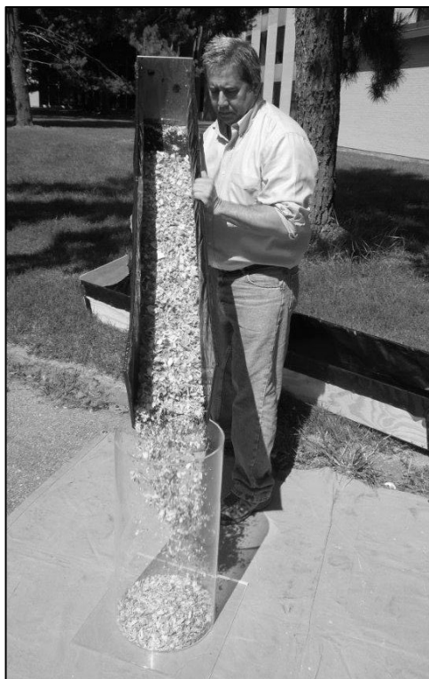
Figure 3-23. Filling a 44 L Test Measure.
