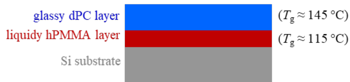
Figure 2. Schematic of the bilayer samples. When the sample is annealed at 130 - 145 °C, the d PC is in the sluggish glass transition state and the h PMMA is in the liquidly melt state.
