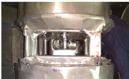
JCNS PASTIS on NEAT showing the cryostat and  $^3\text{He}$  PASTIS cell installed providing large scattering angles.
