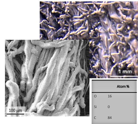
Backcoating Formulation: aluminum hydroxide and silicone - compliant with CA AB2998
