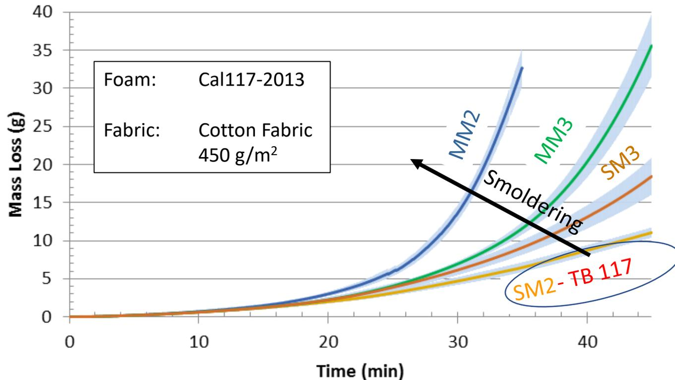
Dynamic mass loss (average and 1 standard Deviation) (3 tests)
