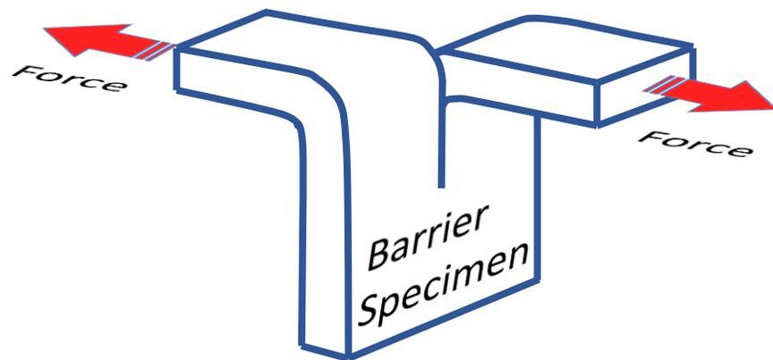
B3 (non-woven oxidized PAN) has a Tear Strength comparable to a letter size paper sheet
