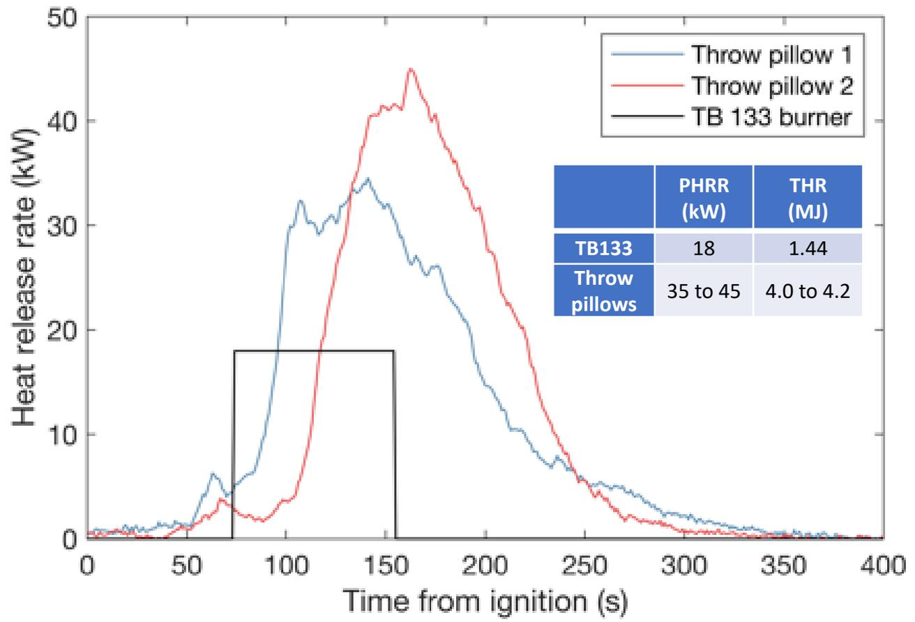
Figure 3: HRR generated by: (1) TB 133 burner and (2) throw pillows
