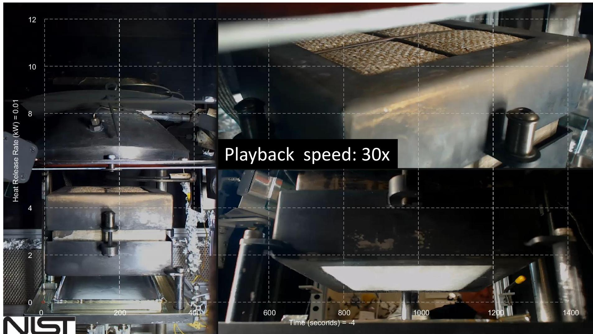
**“Wetting”**: appearance of visible liquid pyrolyzates on the bottom barrier
