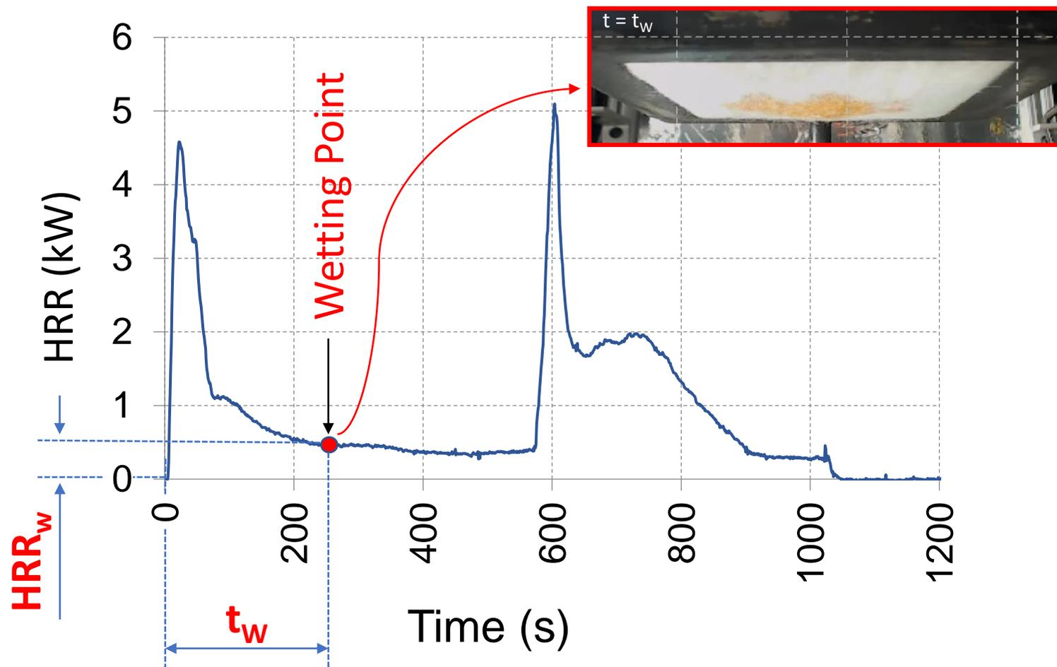
$t_w$  = time to foam liquefaction + time for liquid percolation
