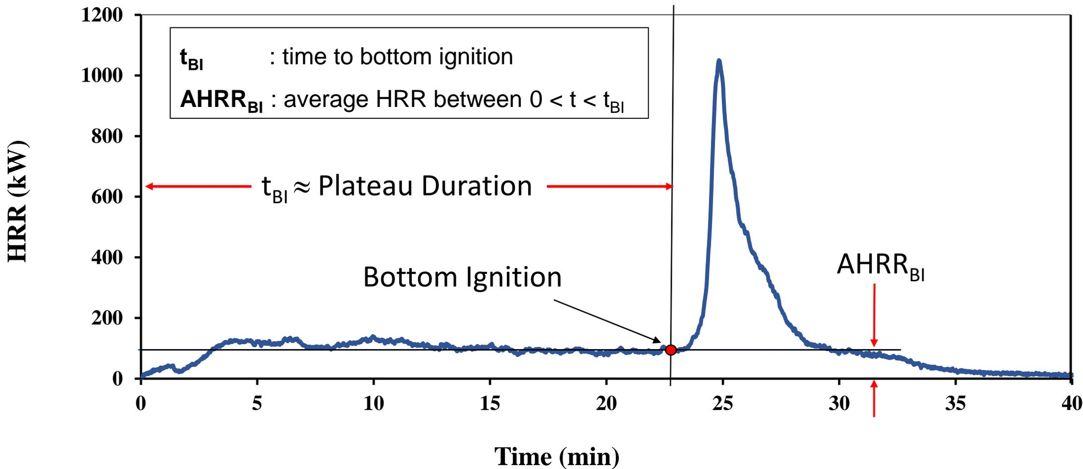
$t_{BI}$  and  $AHRR_{BI}$  are used to characterize "Plateau Phase" burning stage
