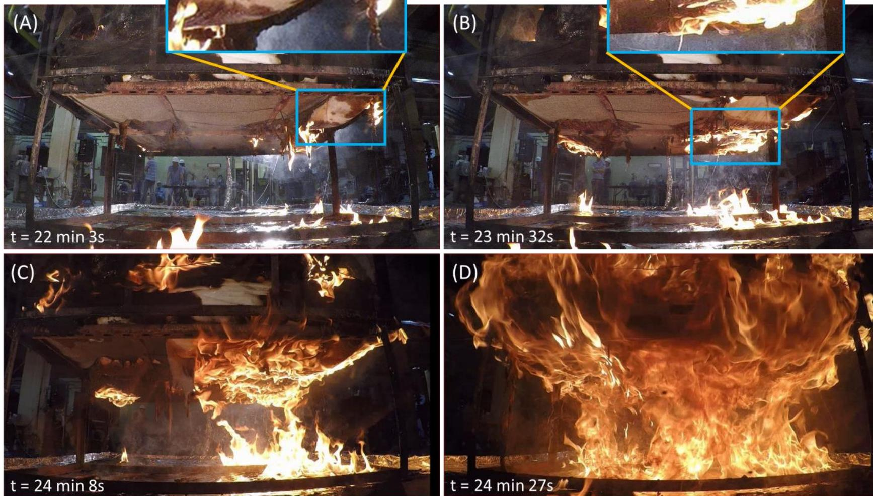
A, **“wetting”** of the barrier due to the percolation of liquid products; B, ignition of liquid products (**“bottom ignition”**); C, pool fire formation, and; D, feed-back between the flame on the pool fire and the remaining fuel in the chair mock-up at the time of PHRR<sub>2</sub>. (Snapshots from Chair B6)
