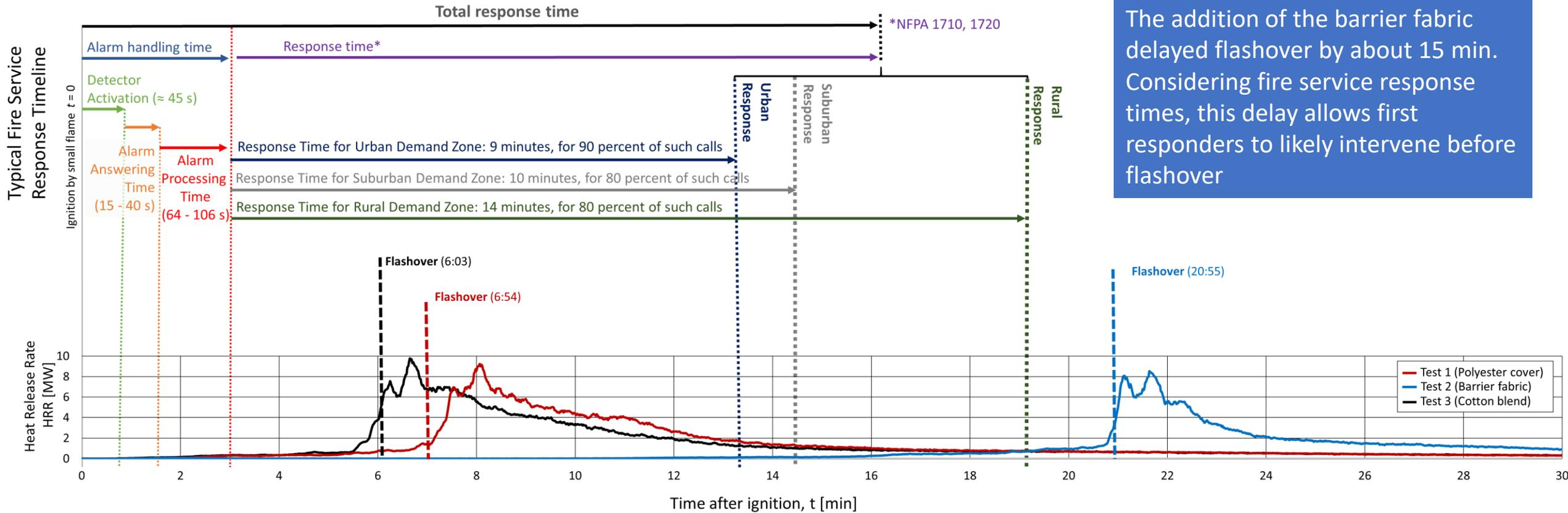
The addition of the barrier fabric delayed flashover by about 15 min. Considering fire service response times, this delay allows first responders to likely intervene before flashover
