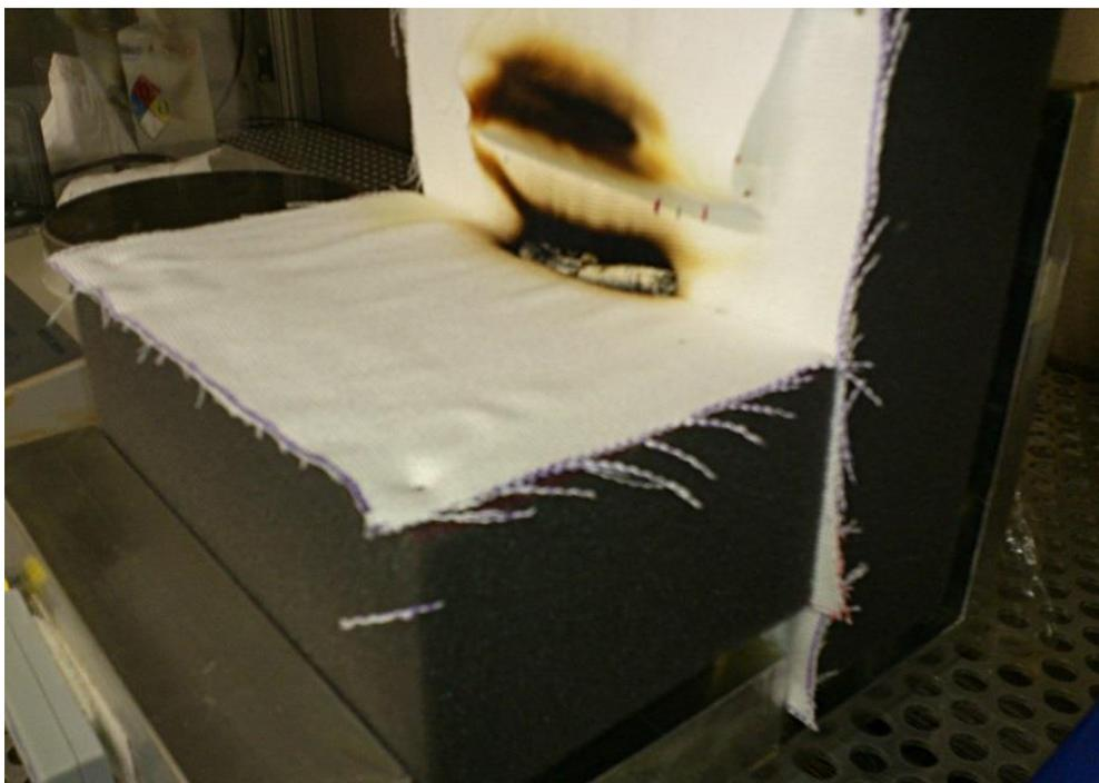
No obvious ignition (smoke or glowing generation) at the end of the 45 min test duration
