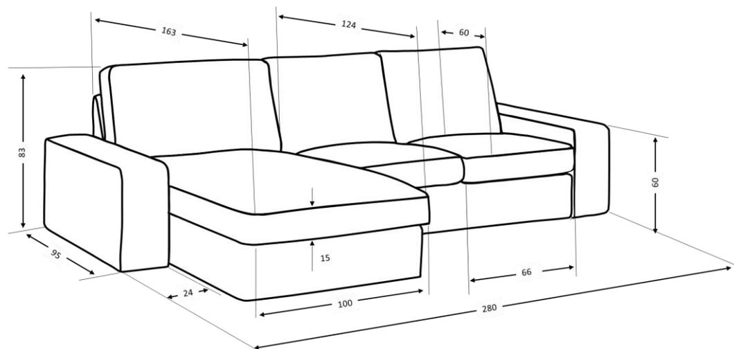
Schematic drawing of the couch (dimensions are in cm)
