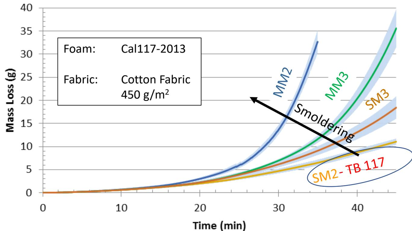
Dynamic mass loss (average and 1 standard Deviation) (3 tests)
