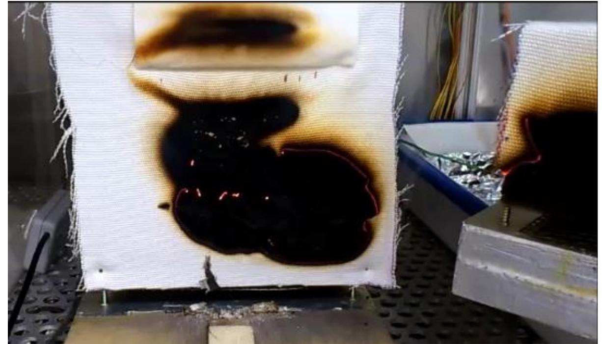
Obvious glowing and smoke generation inside the crevice when the two panels are separated at the end of the test.
