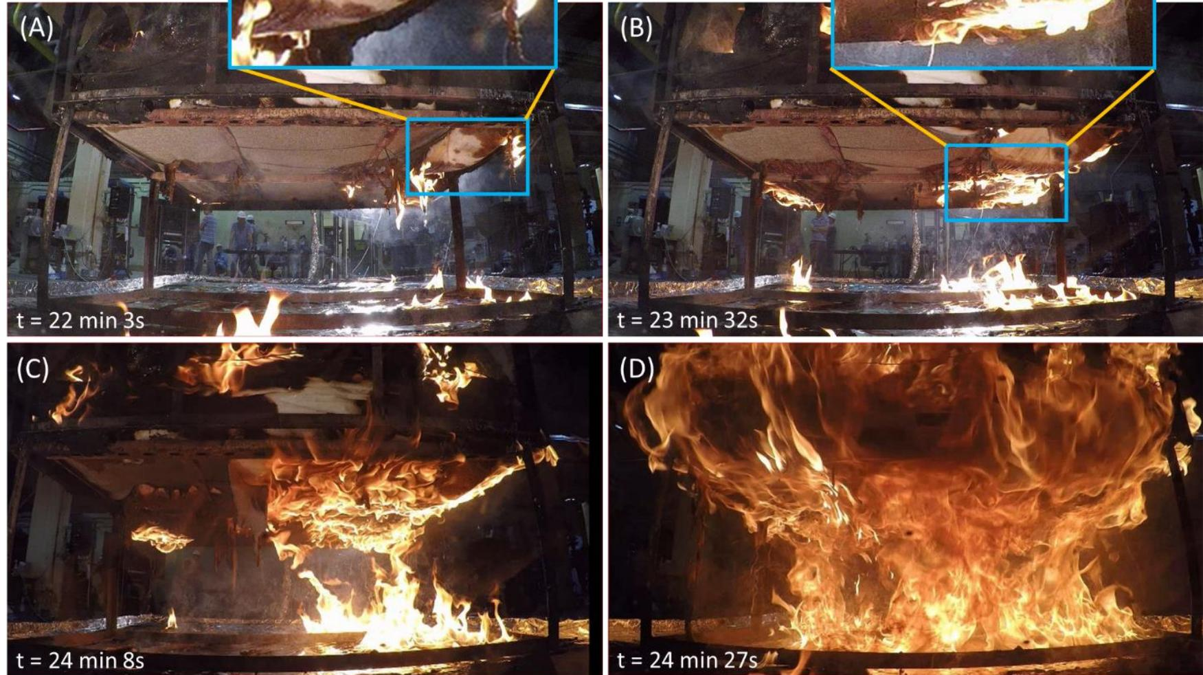
A, **“wetting”** of the barrier due to the percolation of liquid products; B, ignition of liquid products (**“bottom ignition”**); C, pool fire formation, and; D, feed-back between the flame on the pool fire and the remaining fuel in the chair mock-up at the time of PHRR<sub>2</sub>. (Snapshots from Chair B6)
