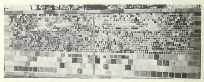
A test wall, comprised of 2352 samples of building stone supplied by 47 states in the U.S.A. and 47 foreign countries, was constructed on the Bureau grounds in 1948 to study the nature and rate of deterioration of the different stones. Structural features such as length changes, warpage, back waterproofing, and grade waterproofing were also observed in relation to weathering and discoloration.
