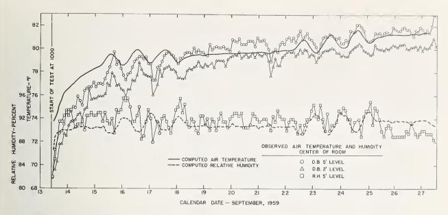
A comparison of the temperatures and humidities observed in an experimental family-size underground shelter during a simulated 2-week hot spell in Washington, D.C., with temperatures and humidities calculated by a finite-difference time-iteration solution of the 3-dimensional heat conduction equation using a digital computer.
