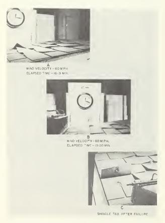
Storm test sequence showing failure of asphalt shingles sealed with plastic cement after exposure to a 60-mph wind in a laboratory storm test machine.
