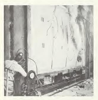
Fire endurance test of a prefabricated lightweight wall panel designed for use in arctic regions. This photograph shows the unexposed surface 55 minutes after the fire exposure started and shortly after flames broke through a joint. Initial failure, at 45 minutes, was due to excessive temperature rise as measured by thermocouples mounted under asbestos pads. The panel continued to support the structural load, applied by jacks at the bottom, throughout the duration of the test.
