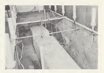
Heat and moisture transfer processes in insulated underground heat distribution systems were studied to find methods of alleviating accelerated pipe corrosion, deterioration of the insulation, and excessive heat loss to the earth. In the photograph, a series of thermocouples is shown affixed at the midlength of an insulating concrete envelope to measure temperature distribution, and standpipes at either side were used to adjust the water table level by introducing water at the bottom.
