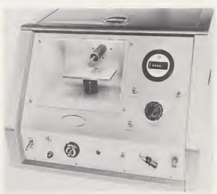
A jet abrader developed at NBS for measuring abrasion resistance of protective coatings. A jet of fine aluminum oxide is projected by pressurized carbon dioxide from the fitting in the upper center of the instrument against the coated specimen below. The time required for the abrasive to penetrate the coating is read from the instrument in the upper right of the cabinet.
