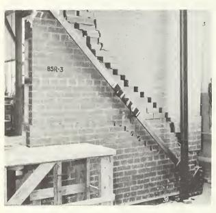
A typical zigzag path of failure of the bond between the mortar and individual masonry units of a composite wall subjected to a racking load.
