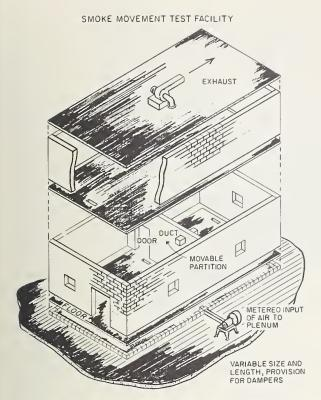
This two-story test facility of brick was designed to permit the study of the spread of smoke and fire both horizontally and vertically under various conditions of ventilation and air flow pattern. The facility has a ventilated plenum under the first floor, floor register openings through the first and second floors, an interior partition and several window openings on the first floor, and an exhaust blower in the second floor ceiling to permit a variety of air flow patterns to be sim-
