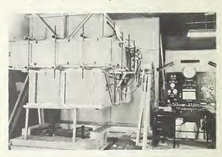
Trunnion-mounted guarded hotbox for measuring heat transmission coefficients of wall, floor, ceiling, or roof constructions. Photograph shows test panel in horizontal position with hot metering box on the bottom and cold box on top indicating heat flow upward as in a ceiling construction. Control panel and instrumentation for observation of test results are shown at the right.
