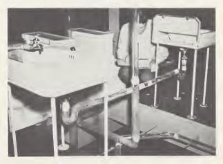
To aid in formulating a Uniform Plumbing Code, complete home plumbing drainage systems of transparent pipes and fittings were constructed in order that the flow phenomena could be observed and photographed.
