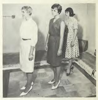
Measurement of the impact noise produced on coverings for concrete floors by footfalls. The sound transmitted to the room below was compared with that produced by a standard tapping machine used in laboratory tests.
