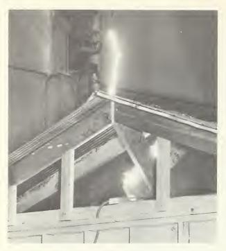
The lightning hazards of ungrounded metallic roofing, siding, and reflective insulation were investigated using high voltage discharges to typical simplified building constructions.
