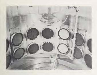
Specimens of organic protective coatings are mounted on the interior periphery of a carbon-arc weatherometer for study of accelerated weathering. The carbon arc, shown in the upper center, is a radiation source used to simulate solar radiation; and the spray nozzles at the right are used to simulate rain.
