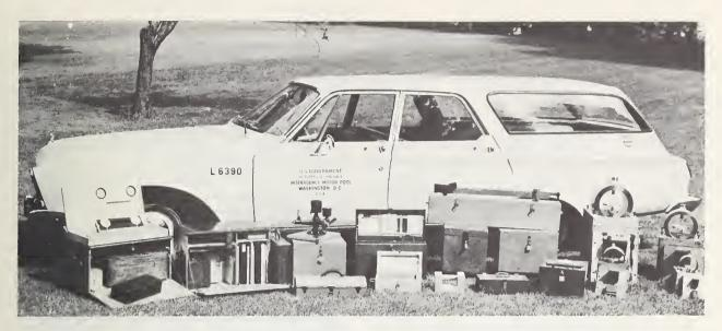
The equipment employed by the NBS Cement and Concrete Reference Laboratory, sponsored by ASTM, to check test methods and apparatus used in cement and concrete testing laboratories throughout the United States and Canada.
