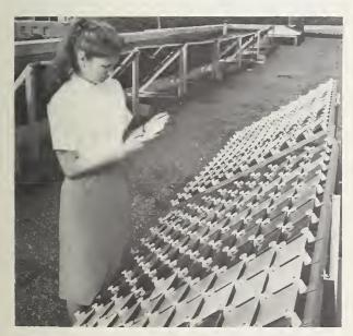
Exposing porcelain enamels on aluminum to determine durability is part of a current program to develop standard test procedures for porcelain properties such as weather resistance, alkali resistance, and ease of cleaning.
