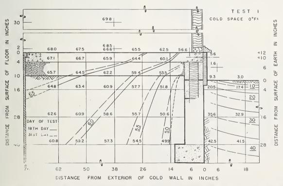
Temperature patterns and isothermal lines under winter conditions in a concrete floor slab construction laid over gravel and earth with insulation applied at the edge of the floor and foundation. The upper and lower figures show the temperature distributions under sustained outdoor temperatures of 32 °F and 0 °F, respectively.
