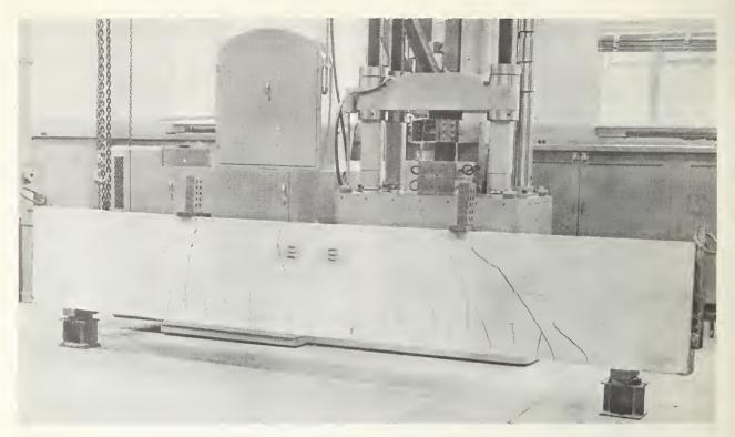
A typical crack pattern for a reinforced concrete beam is shown in this test specimen. Control of the width of cracks is an important factor in the design of reinforced concrete structures since crack width is related to the integrity and economy of reinforcement. Theoretical analysis and experimental study at NBS of the principal factors controlling the spacing and width of cracks in concrete beams have contributed to design practice.
