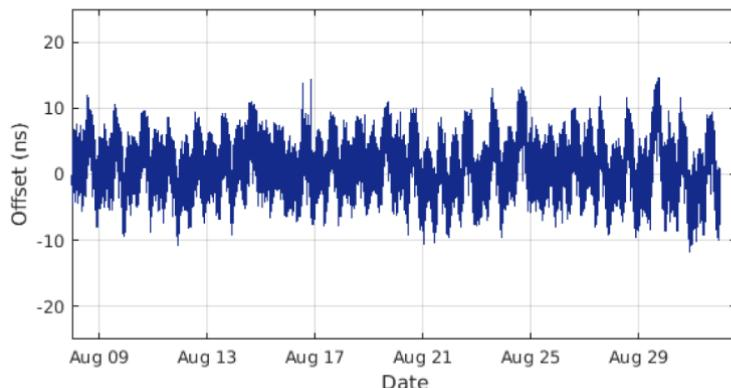
In the case of any kind of service disruption detected at the client site, the customer equipment holdover guarantees a time drift below 1.5 microseconds after 24 hours.
