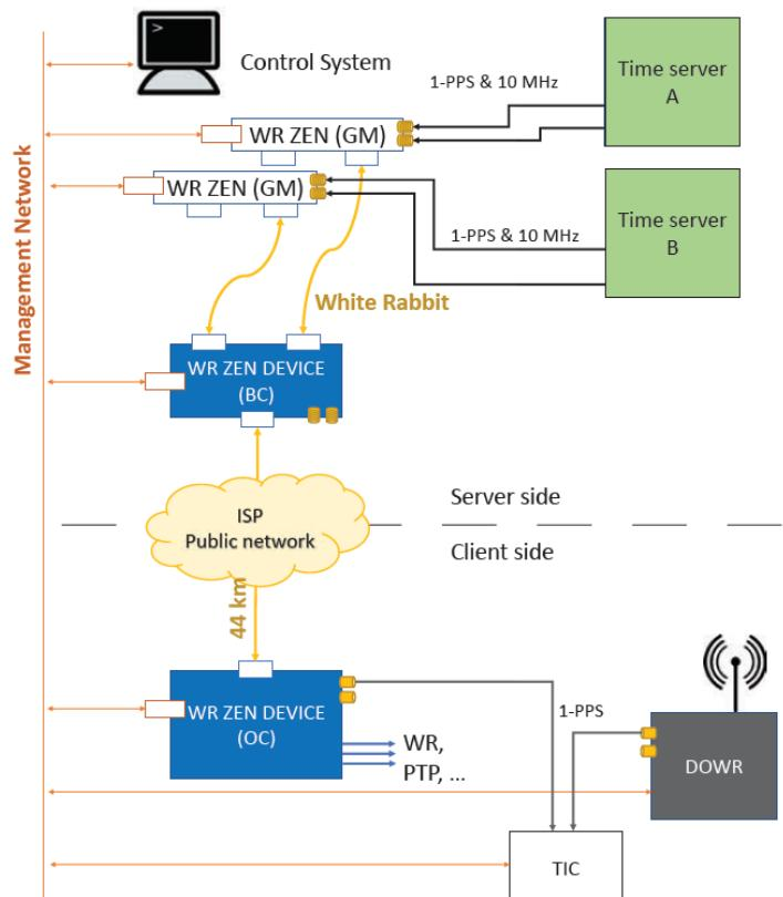
At the customer side, a **WR-ZEN** is synchronized to the time server through a White Rabbit link and it provides the customer with time signals over different protocols for interoperability with other elements at the end nodes.
