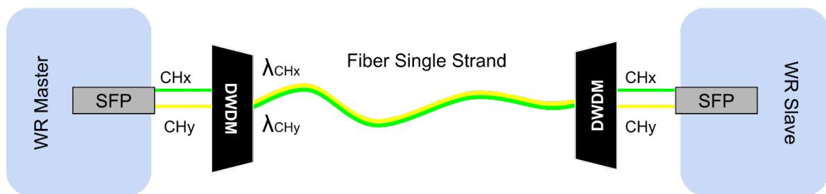
This deployment allows to deploy a plug-and-play long-distance White Rabbit link using pre-calibrated values up to 100 km without amplification.
