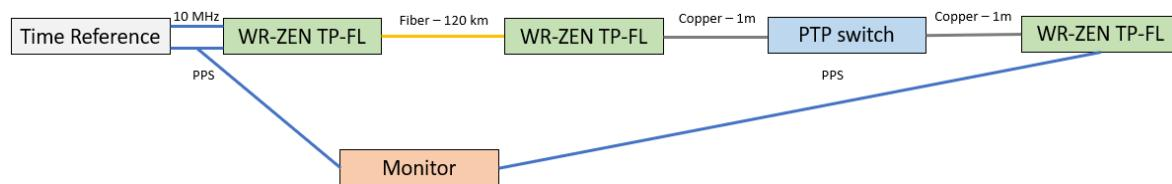
In the framework of **telecommunication** networks, packet-based synchronization is used for timing dissemination to reduce the GNSS dependency, the associated costs and to improve timing performance. In example, Fifth Generation (5G) technologies demand more strict synchronization requirements between 110 and 12.5 nanoseconds and, at the same time, require advanced capabilities related to reliability and redundancy.
