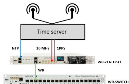
If the time server does not support these capabilities, two WR-ZEN TP devices can be used to get the time references and a WR-switch that can be manually configured to switch from a primary to a backup time reference.
