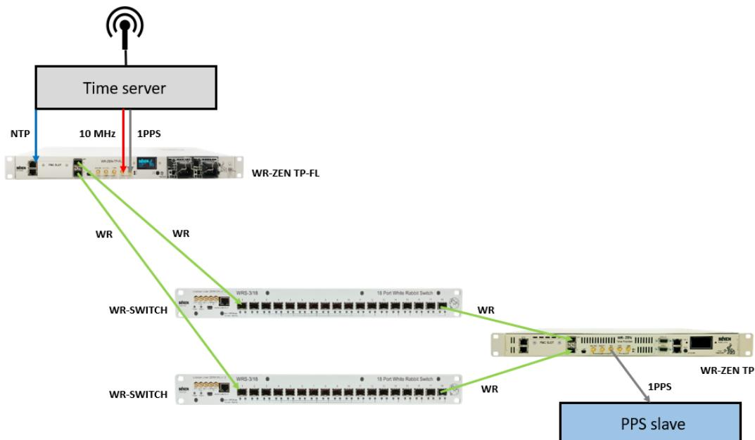
Additionally, a second WR-ZEN TP can be deployed as last White Rabbit device to feed a PTP switch or slave that implements Best Master Clock Algorithm
