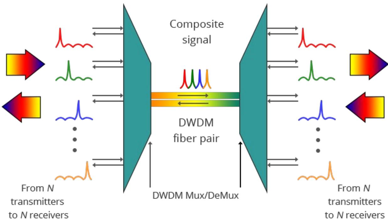
This topology leads to an asymmetry issue because of different latencies in the fiber paths. This asymmetry can be removed combining pre-calibration of the used optical components and specific link calibration.
