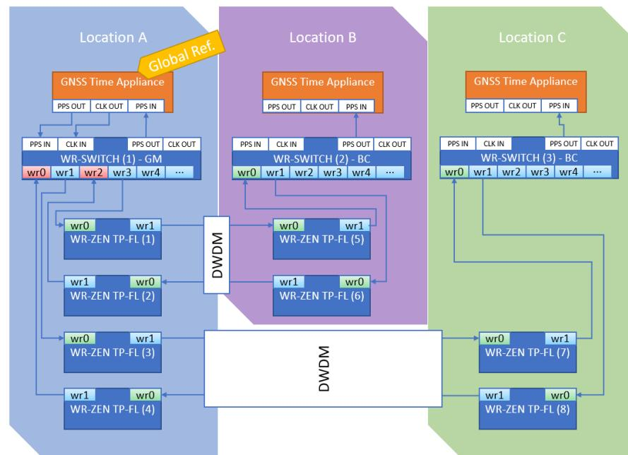
Remote time signal backup based on a time server
