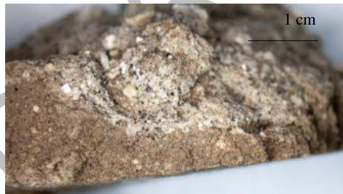
FIG. 7: A soil sample with multiple layers evident. Care should be taken during packaging to preserve the layer structure during shipping/transport from the field to the laboratory. Photograph courtesy of Marianne Stam.
