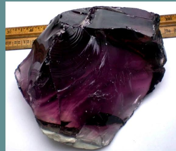
Glass produced from a high level radioactive waste simulant
