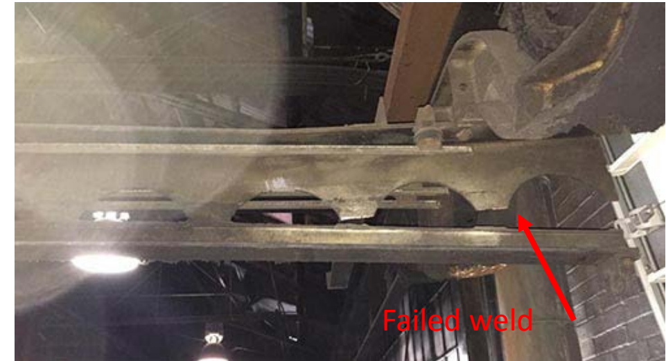
Example of a failed arch beam crane from the web—this is not a picture of a NIST crane.
