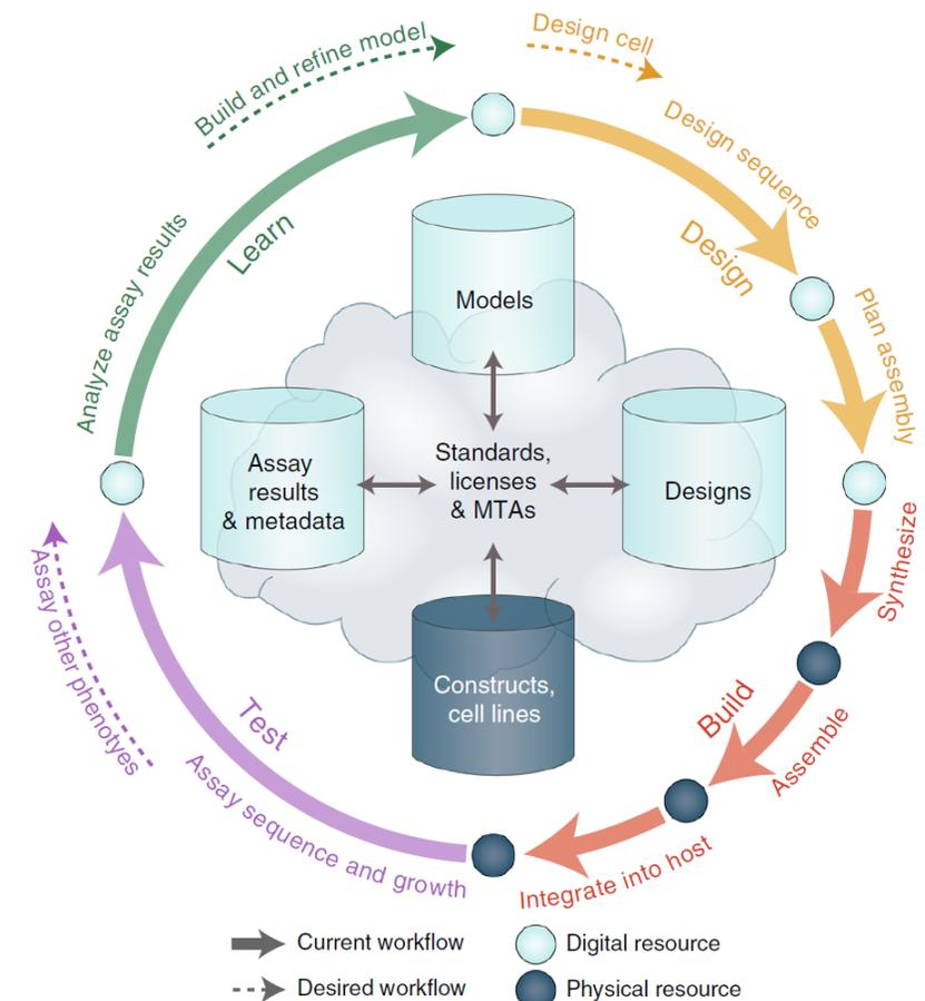
**Fig. 2** The emerging design-build-test-learn workflow for genome engineering is shown schematically with current (solid arrows) and likely future (dashed arrows) tasks, interfaces (circles), and repositories (cylinders), either digital (light) or physical (dark).
