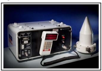
Around the same time, scientists at the NASA Jet Propulsion Laboratory developed the technology that led to the development of the Macrometer Interferometric Surveyor. Thus, several federal agencies played an important role in transferring the technology that led to the first commercial GPS receivers, and the legacy is that most features from these early models are found in GPS receivers today.
