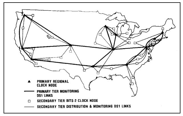
Figure 4-1. AT&T Verifiable Digital Sync Plan
