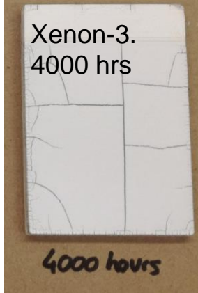
Xenon-3: High Irra, High T, Low RH, Water spray
