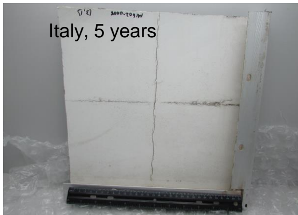
Xenon-3: High Irra, High T, Low RH, Water spray
