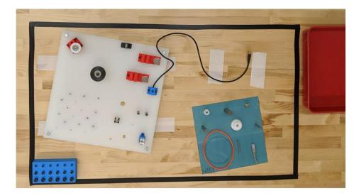
Figure 4: Layout for assembly-subtask 2 showing task board and kit layout with a method of dispensing screws.
