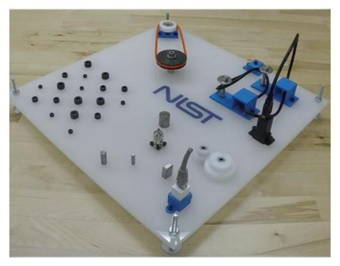
Figure 1: Fully assembled practice task board
