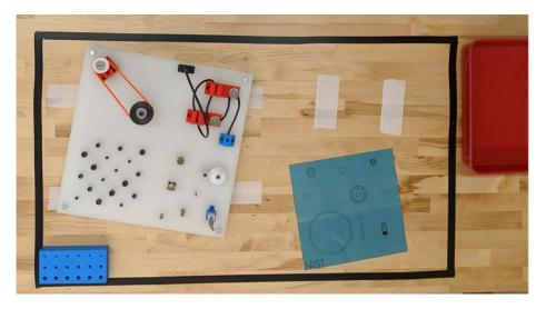
Figure 5: The practice task board will all parts successfully assembled.
