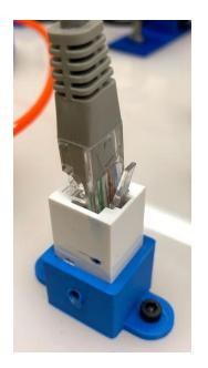
Insertion into mating counter part but no snap fit of locking mechanism (3 points)
