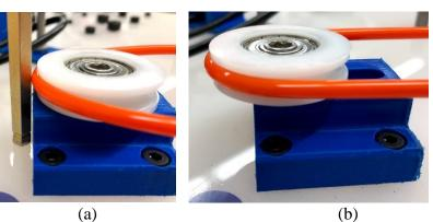
Belt outer diameter aligns or protrudes back surface of slide tensioner bracket as shown in (a) and (b) - (14 points)
