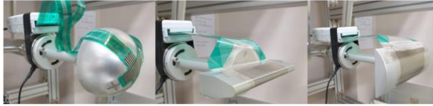
Fig. 2: Three shapes of impactor with pressure measuring film (left: 40 mm radius hemisphere, center: cylinder edge of 5mm radius, right: cylinder edge of 40 mm radius)
