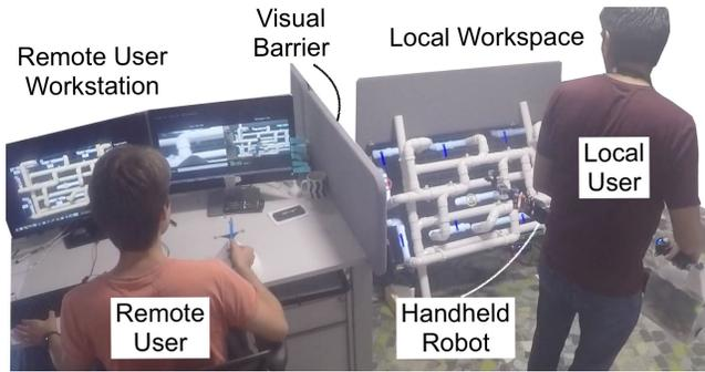
Fig. 2: Overview of the remote assistance experiment setup. A remote user controls the semi-autonomous handheld robot to support the local user in the workspace.
