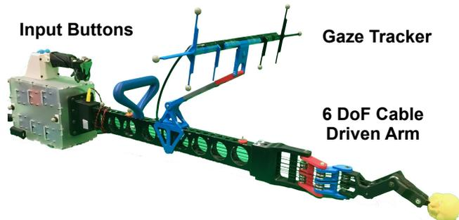
Fig. 1: Handheld robot with extended user perception capabilities through a newly integrated eye tracking system.
