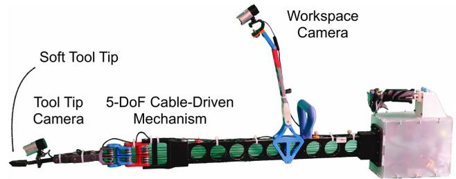
Fig. 3: Handheld Robot with remote-controlled 5-DoF tooltip and equipped cameras and a tooltip for sensor simulation .
