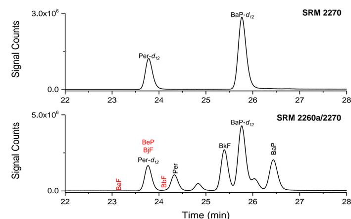
Figure 2: RPLC/FL chromatograms obtained using the separation conditions in Table 1. The red labels refer to the four additional MM 252 PAHs present in SRM 2260a.
