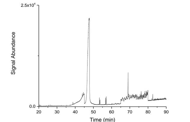
Figure 5: GC/MS chromatogram in SIM mode for the spiked olive oil sample after SEC fractionation.
