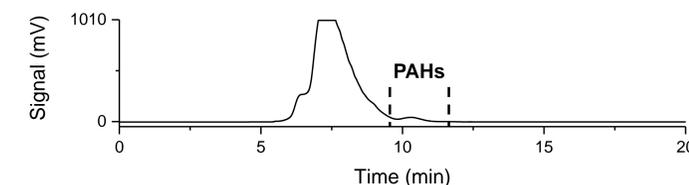
Figure 3: SEC fractionation chromatogram of spiked olive oil sample.
