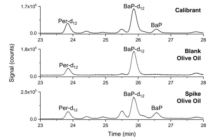
Figure 4: RPLC/FL chromatograms obtained for the calibrant, blank olive oil, and spiked olive oil samples after SEC fractionation.
