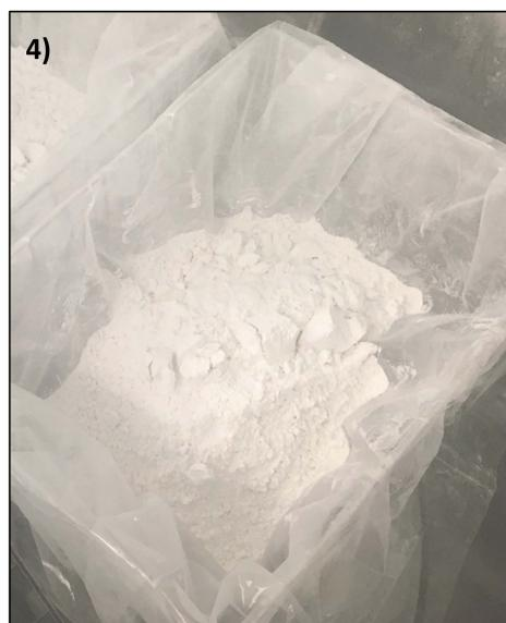
4.) Cryohomogenized powder sample falls from a distribution tube at the bottom of the Cryomill. The sample is caught in a container and quickly placed in an LN<sub>2</sub> vapor-phase freezer (-150° C).
