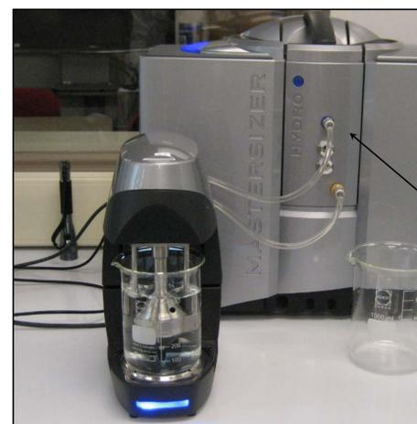
Particles are recirculated via wet dispersant. Lasers produce scatter as particles pass through beams. Light scattering and optical properties of the material are used to determine the equivalent spherical diameter.
