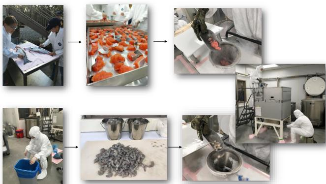
○ Materials were cryohomogenized three times using a Palla VM-KT Vibrating cryomill, generating a fine fresh-frozen powder
