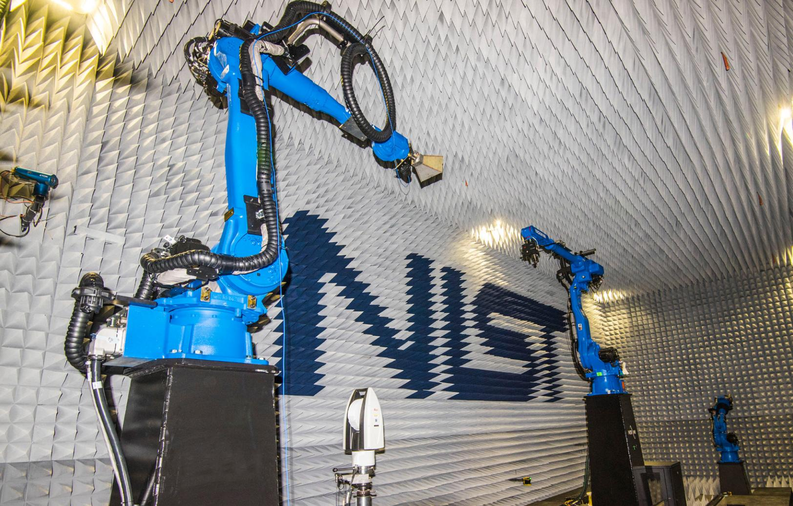
The NIST Antenna Metrology Project performs measurements on advanced antenna systems operating in complex environments. For example, the Large Antenna Positioning System (pictured) is supporting the development of next-generation 5G wireless and spectrum sharing systems.
