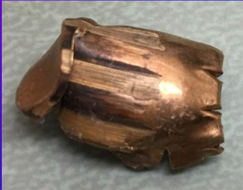
Metal jacket is **detached** from the lead core. Pliers were used to bend the jacket to make it measurable.
