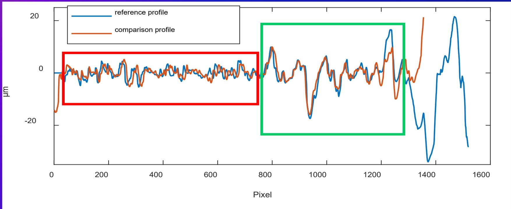
The **maximum overall similarity value (using normalized CCF)** between the reference and comparison profiles is **only 0.43**.
