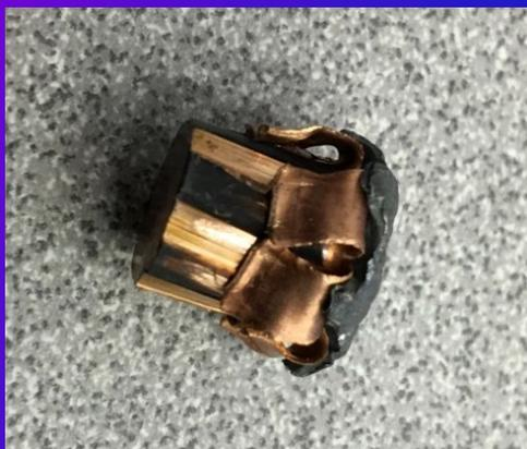
Metal jacket adheres to the lead core. **Nose area expanded** due to impact.
