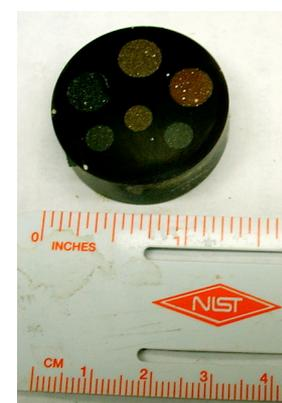
The specimen is polished on the outer portion, and then cleaned of polishing residue in the center of the cloth. There are many different types of polishing cloths and plates, I use these cotton SEM cleaning cloths, which are used once and then discarded.
