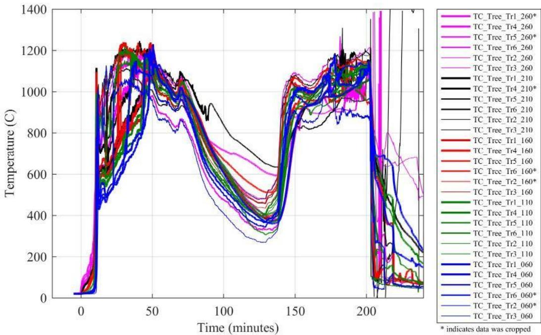
Figure I 8. Thermocouple tree temperatures at various locations inside the compartment.
