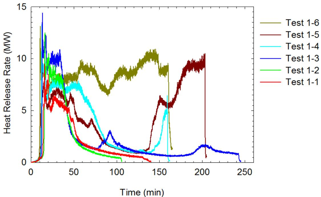
Figure 103. Heat release rates in CLT compartment tests.
