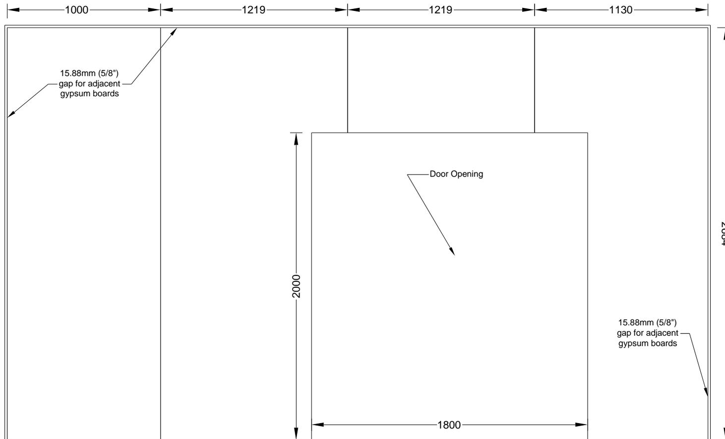
NOTE: 15.88mm (5/8") Type-X Gypsum Board Fastened w/ 41mm (1 5/8") Type-S Drywall Screws Used
