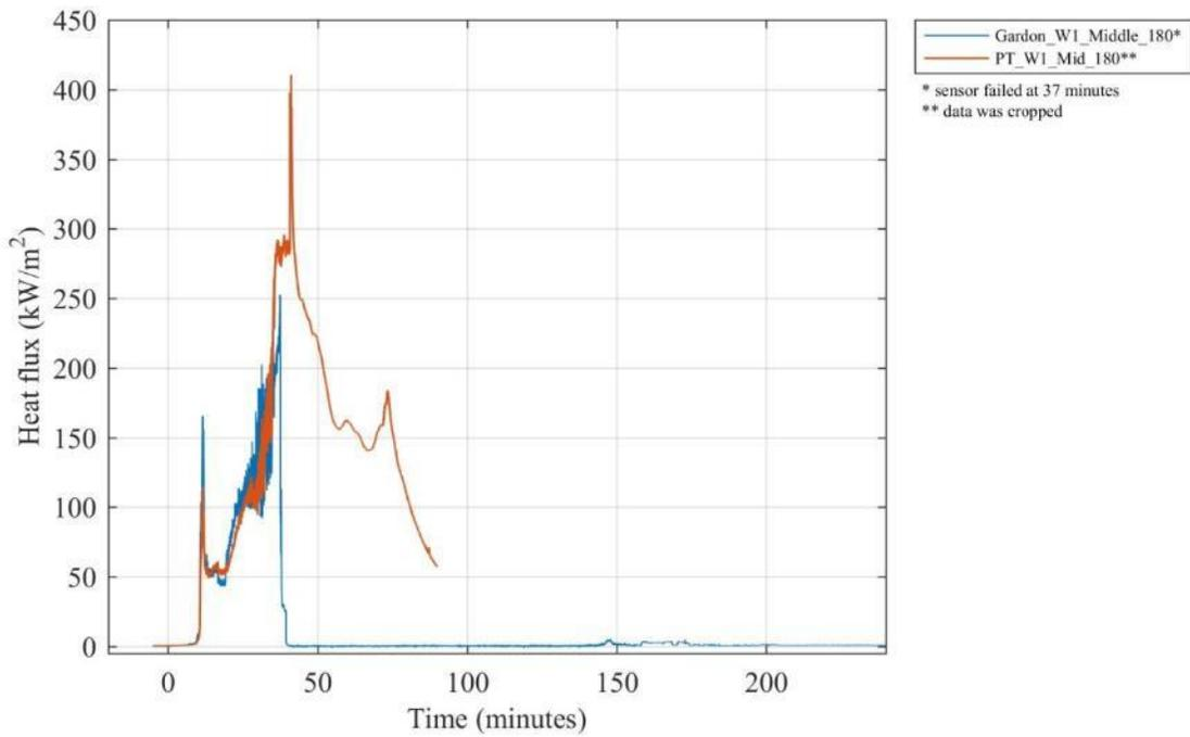
**Figure I 20. Comparison of heat fluxes recorded by a collocated Gardon gauge, plate thermometer (PT) and differential flame thermometer (DFT) on Wall W1 at the middle of the compartment 1.8 m above the floor.**
