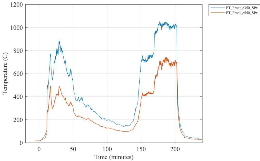
**Figure I 30. Plate thermometer temperatures 350 cm and 550 cm above the floor above the doorway.**
