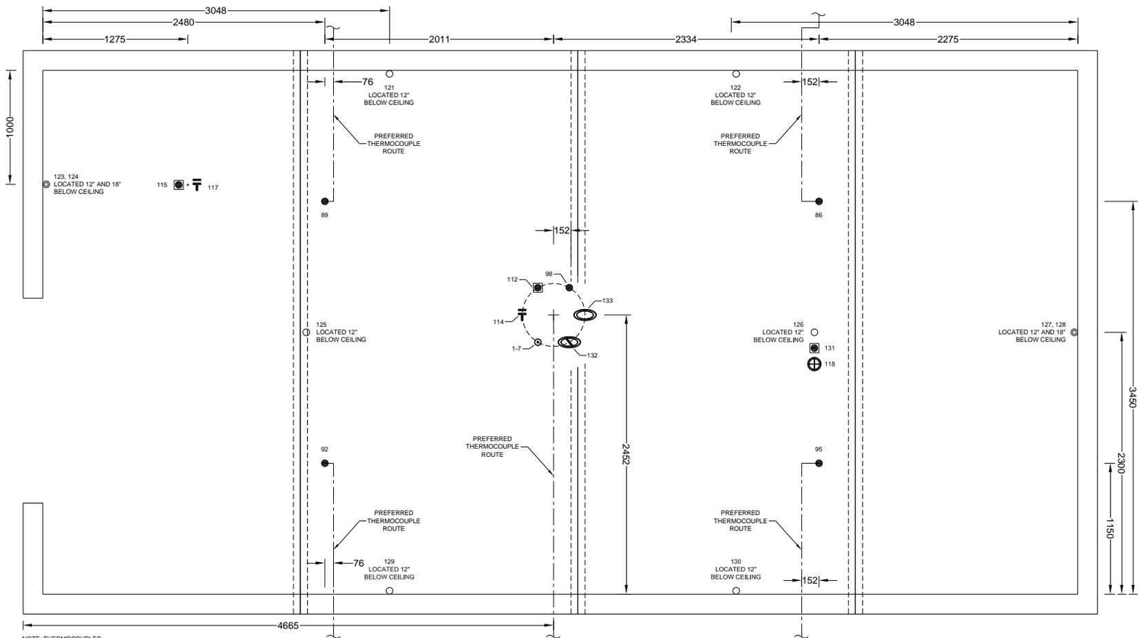
NOTE: THERMOCOUPLES 86, 89, 92, 95, 98 ARE TO BE INSTALLED PRIOR TO GYPSUM WALL BOARD.
