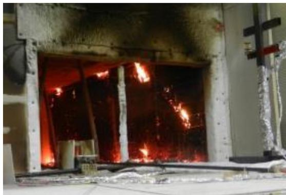
(g) exposed W1 at 240 min after 2<sup>nd</sup> ply falling off
