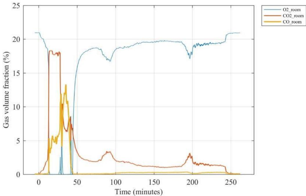
**Figure G 3. Gas volume fractions for oxygen (O<sub>2</sub>), carbon dioxide (CO<sub>2</sub>) and carbon monoxide (CO) sampled at the center of the compartment 210 cm above the floor.**
