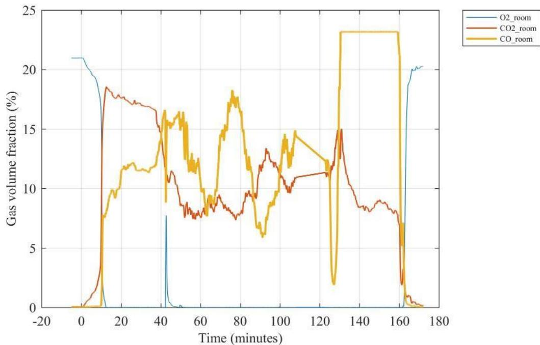
**Figure J 3. Gas volume fractions for oxygen (O<sub>2</sub>), carbon dioxide (CO<sub>2</sub>) and carbon monoxide (CO) sampled at the center of the compartment 210 cm above the floor.**
