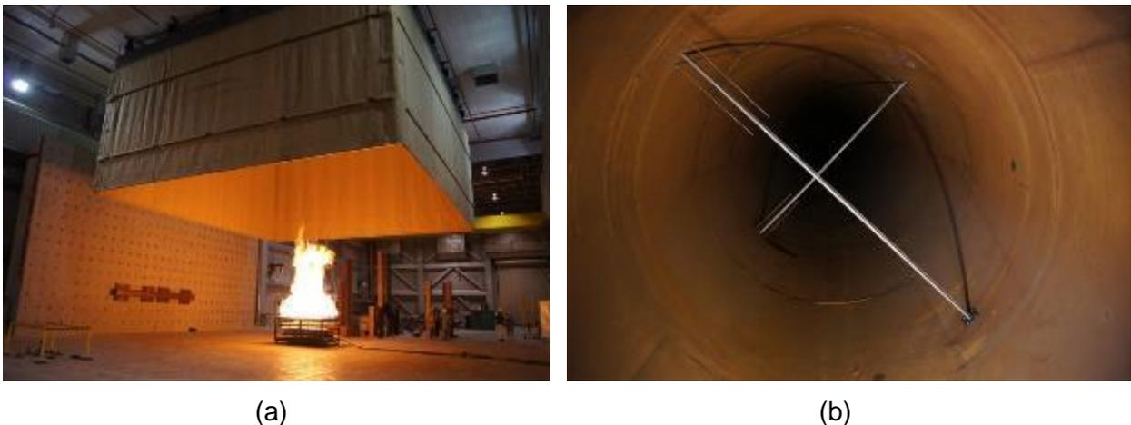
**Figure 29. (a) 15-m exhaust hood with natural gas reference burner at 5 MW and (b) 2.42-m diameter calorimeter exhaust duct with averaging pitot tubes and temperature sensors (gas sample tube not shown).**
