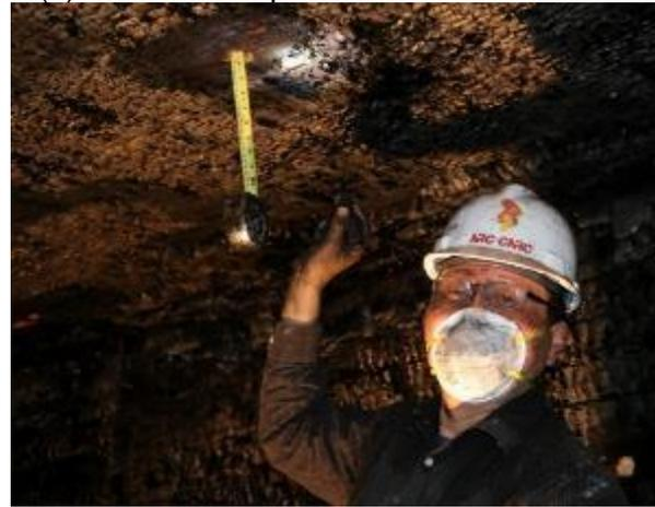
(d) char measurement by drilled holes
