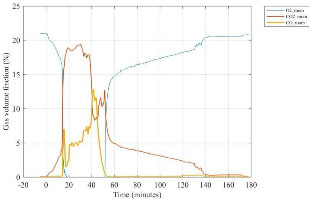
**Figure E 3. Gas volume fractions for oxygen (O<sub>2</sub>), carbon dioxide (CO<sub>2</sub>) and carbon monoxide (CO) sampled at the center of the compartment 210 cm above the floor.**
