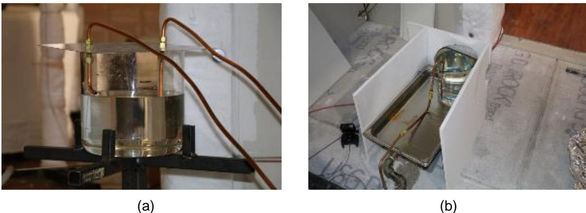
Figure 40. Photographs of water-cooled camera setup (a) 1<sup>st</sup> attempt and (b) improved setup.
