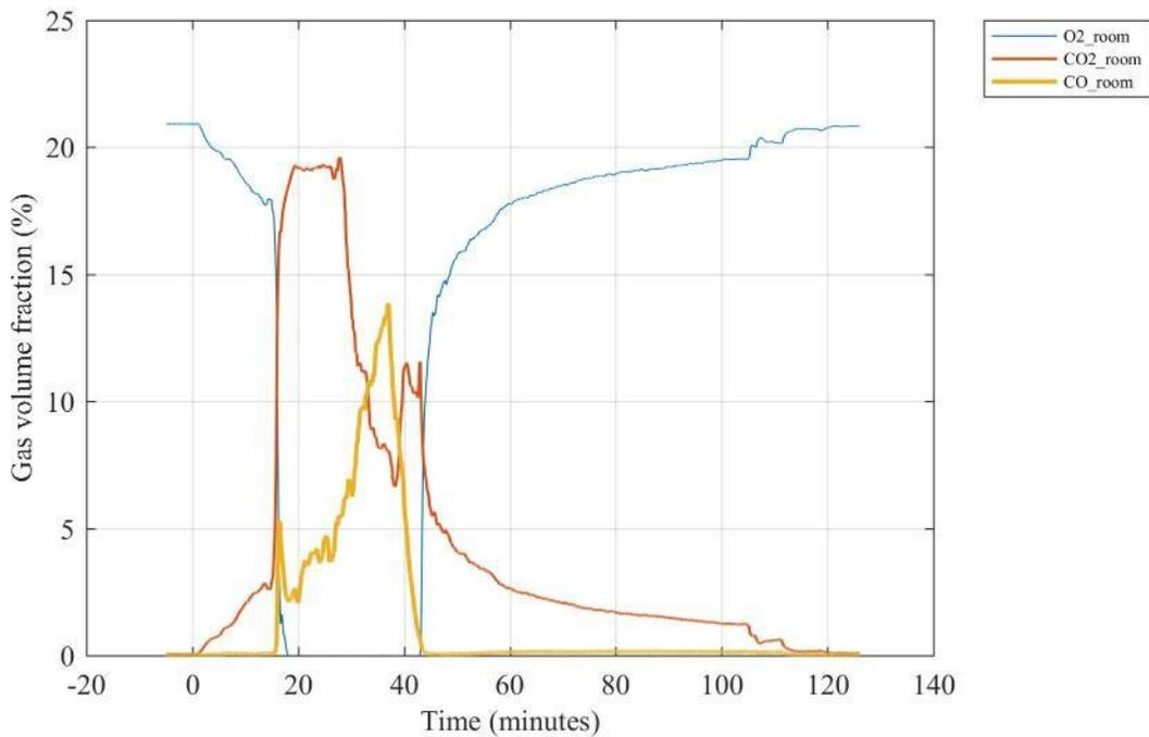
**Figure F 3. Gas volume fractions for oxygen (O<sub>2</sub>), carbon dioxide (CO<sub>2</sub>) and carbon monoxide (CO) sampled at the center of the compartment 210 cm above the floor.**
