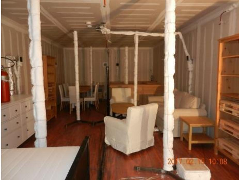
**Figure 13. Photograph of the movable fuel as installed.**
