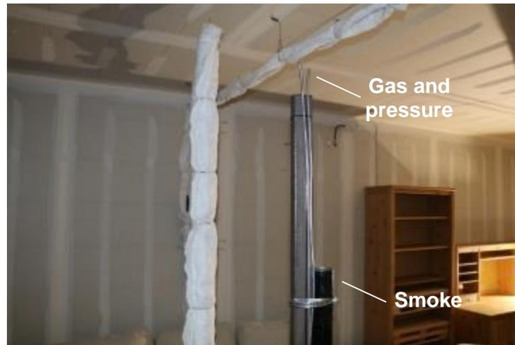
Figure 30. Photograph of stand with gas sampling tubes.
