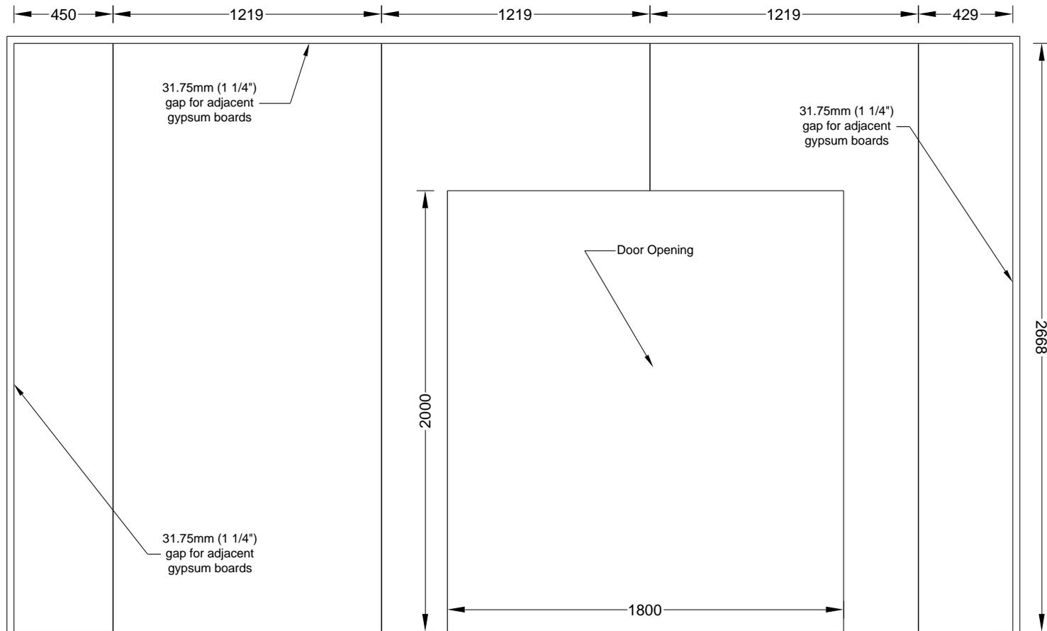
NOTE: 15.88mm (5/8") Type-X Gypsum Board Fastened w/ 57mm (2 1/4") Type-S Drywall Screws Used
