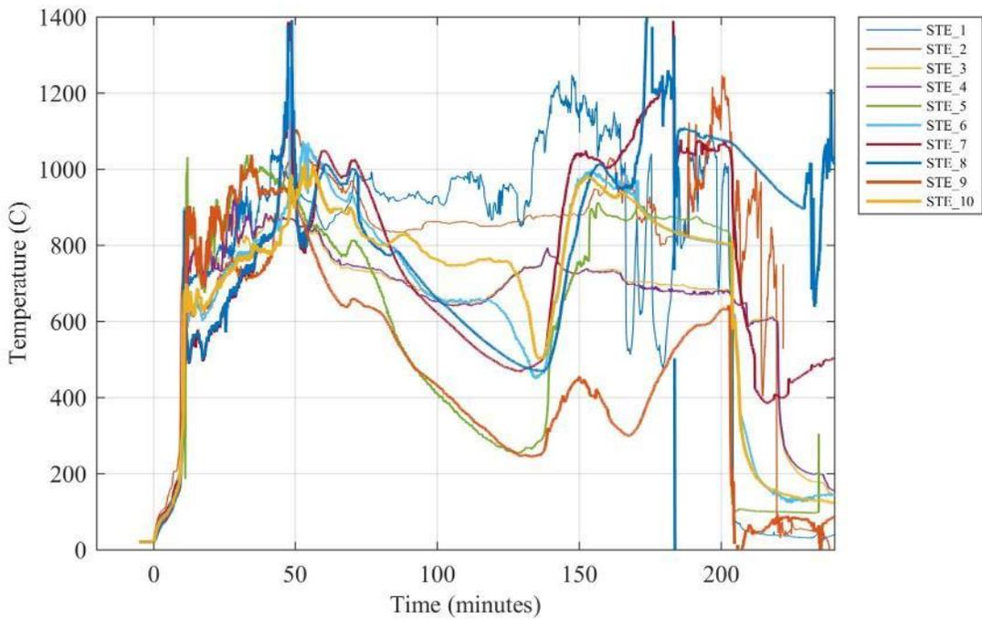
**Figure I 4. Simulated thermal elements (STE) for sprinkler.**
