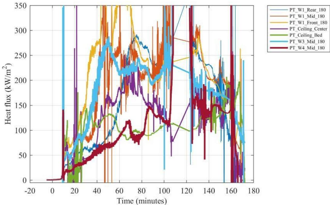
**Figure J 17. Heat flux calculated from plate thermometers at various locations inside the compartment.**
