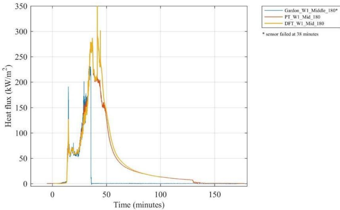
**Figure E 21. Comparison of heat fluxes recorded by a collocated Gardon gauge, plate thermometer (PT) and differential flame thermometer (DFT) on Wall W1 at the middle of the compartment 1.8 m above the floor.**
