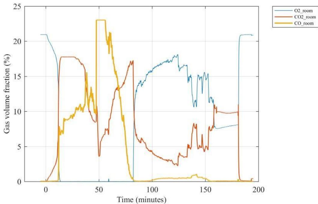
**Figure H 3. Gas volume fractions for oxygen (O<sub>2</sub>), carbon dioxide (CO<sub>2</sub>) and carbon monoxide (CO) sampled at the center of the compartment 210 cm above the floor.**
