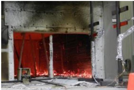
(e) exposed W1 at 120 min after 1<sup>st</sup> ply falling off
