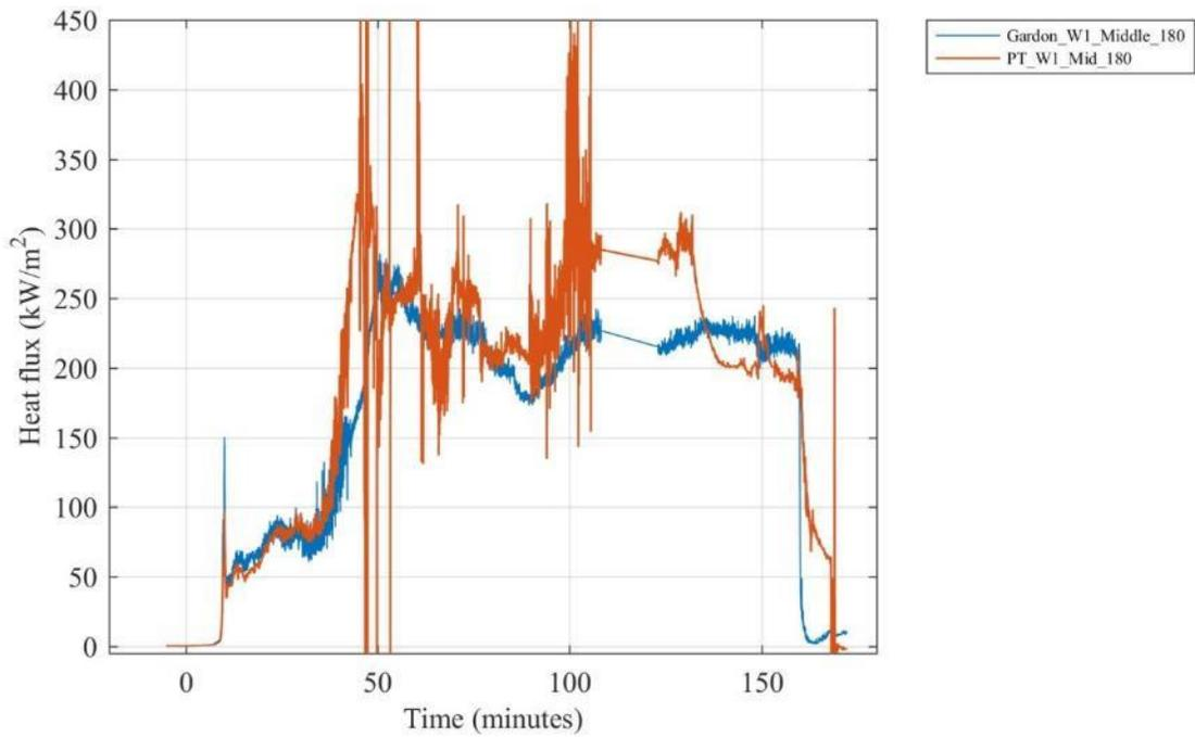
**Figure J 20. Comparison of heat fluxes recorded by a collocated Gardon gauge, plate thermometer (PT) and differential flame thermometer (DFT) on Wall W1 at the middle of the compartment 1.8 m above the floor.**
