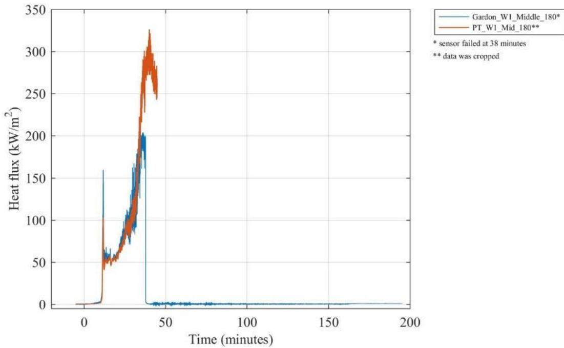
**Figure H 20. Comparison of heat fluxes recorded by a collocated Gardon gauge, plate thermometer (PT) and differential flame thermometer (DFT) on Wall W1 at the middle of the compartment 1.8 m above the floor.**
