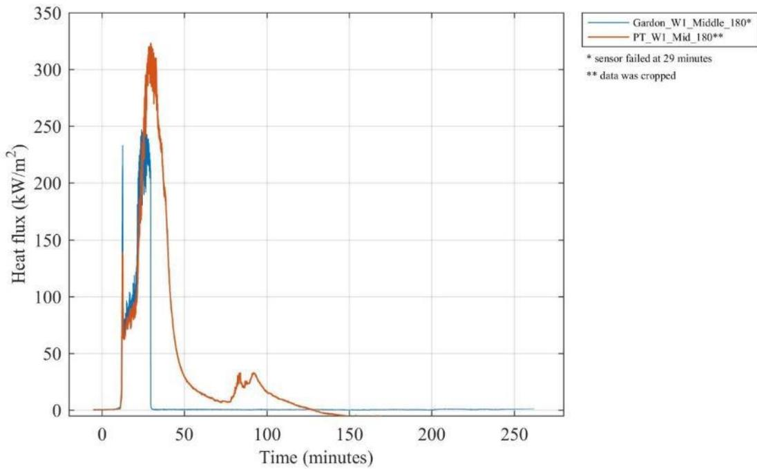
**Figure G 20. Comparison of heat fluxes recorded by a collocated Gardon gauge, plate thermometer (PT) and differential flame thermometer (DFT) on Wall W1 at the middle of the compartment 1.8 m above the floor.**
