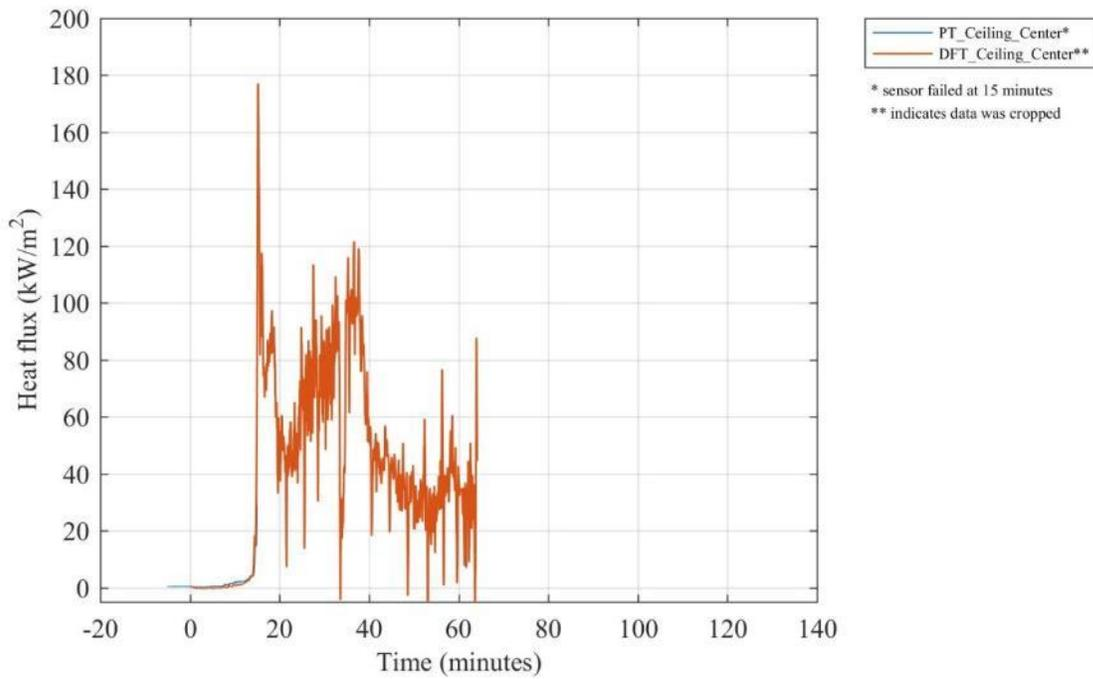
**Figure F 22. Comparison of heat fluxes recorded by a collocated plate thermometer (PT) and differential flame thermometer (DFT) on the ceiling at the center of the compartment.**
