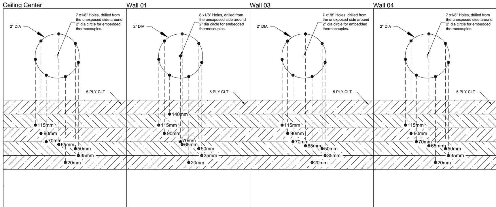
Figure A 86. Test 1-5 Large Compartment CLT - Embedded Thermocouple Detail
