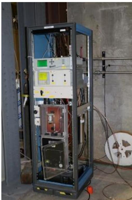
**Figure 31. Photograph of gas analyzer rack.**
