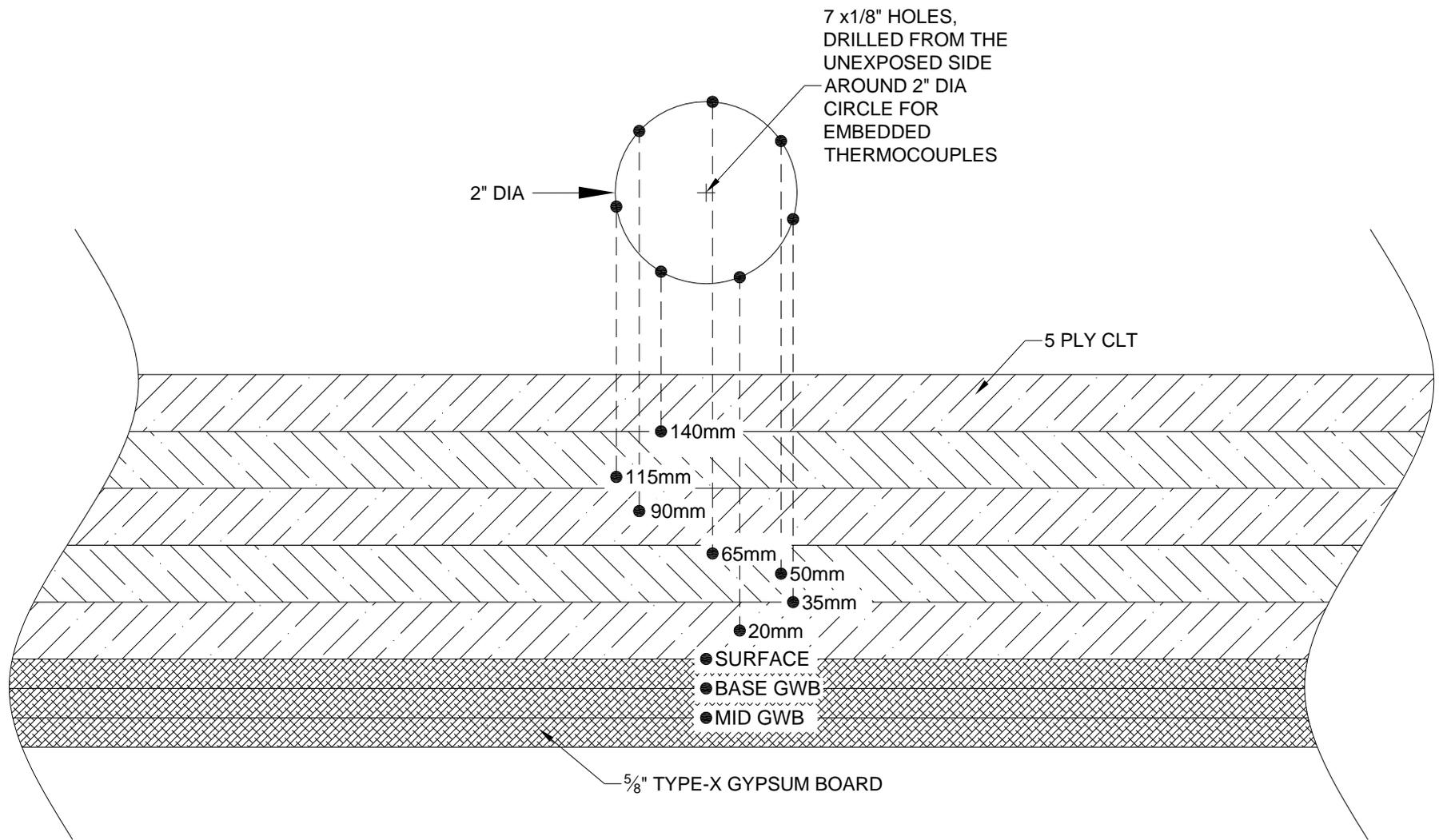
**Figure 26. Details of embedded thermocouples in ceiling and walls with the drilled holes sealed from the outside (additional thermocouples added at the 2<sup>nd</sup> and 3<sup>rd</sup> gluelines in Test 1-5 and Test 1-6).**
