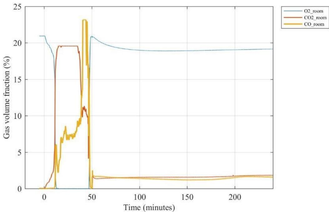
**Figure I 3. Gas volume fractions for oxygen (O<sub>2</sub>), carbon dioxide (CO<sub>2</sub>) and carbon monoxide (CO) sampled at the center of the compartment 210 cm above the floor.**
