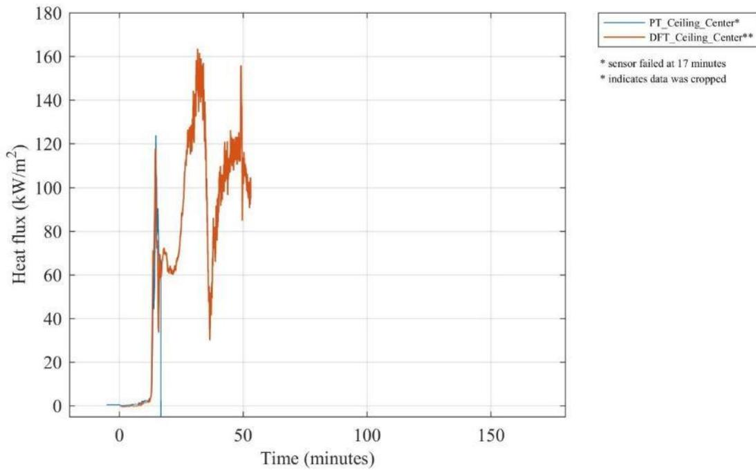
**Figure E 22. Comparison of heat fluxes recorded by a collocated plate thermometer (PT) and differential flame thermometer (DFT) on the ceiling at the center of the compartment.**
