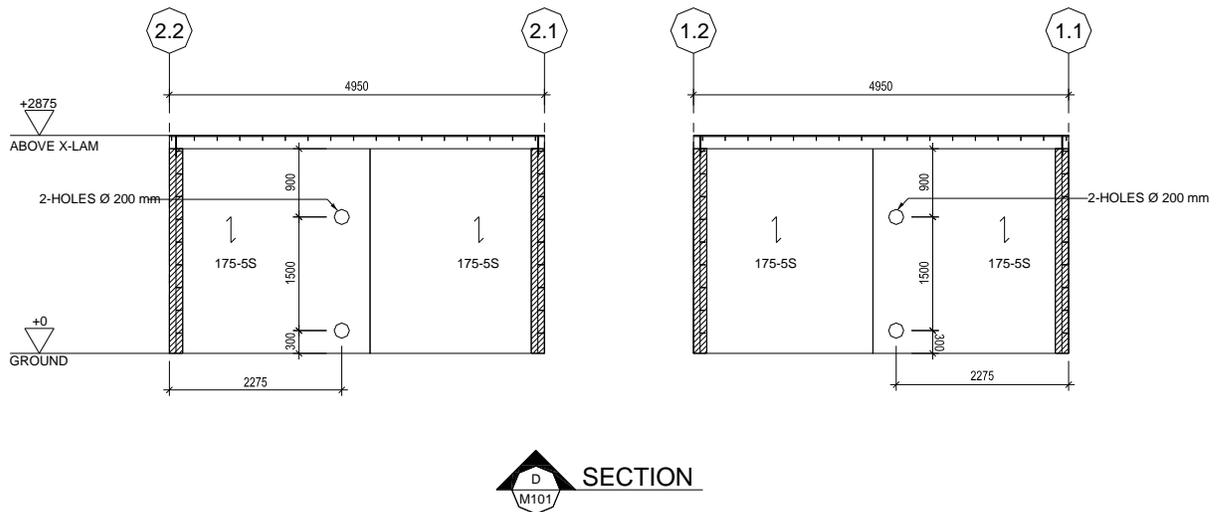
**Figure 4. Elevation and Section View of CLT Compartments.**
