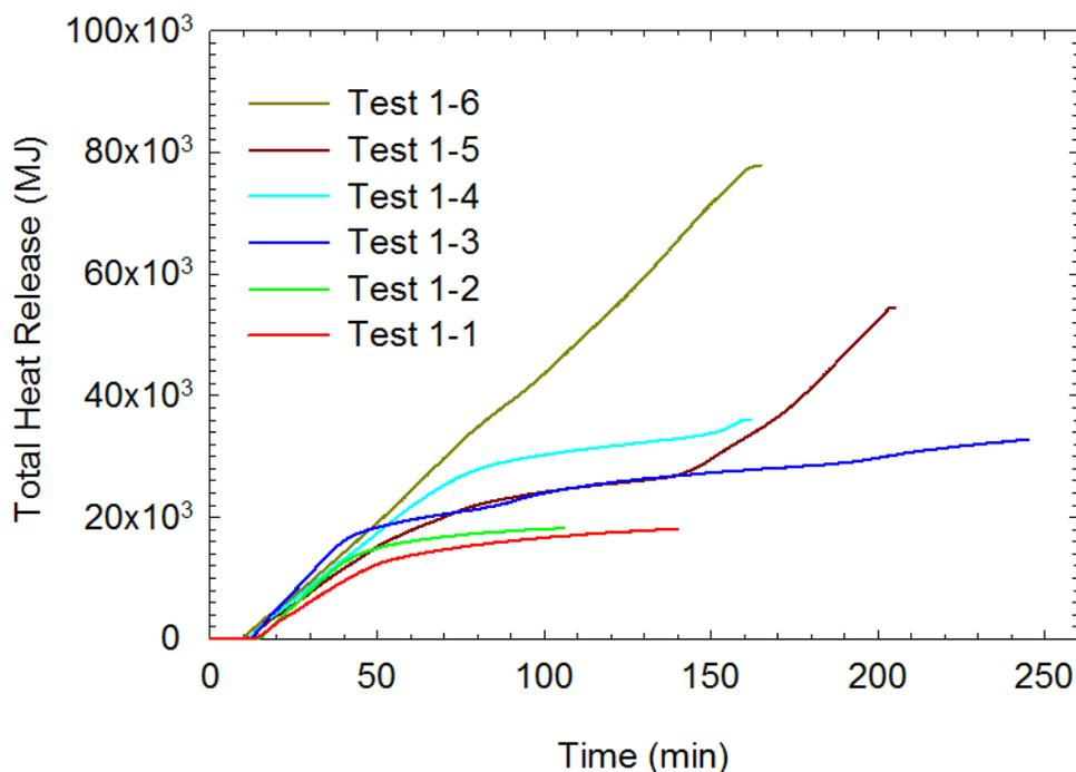
**Figure 104. Total heat releases in CLT compartment tests.**
