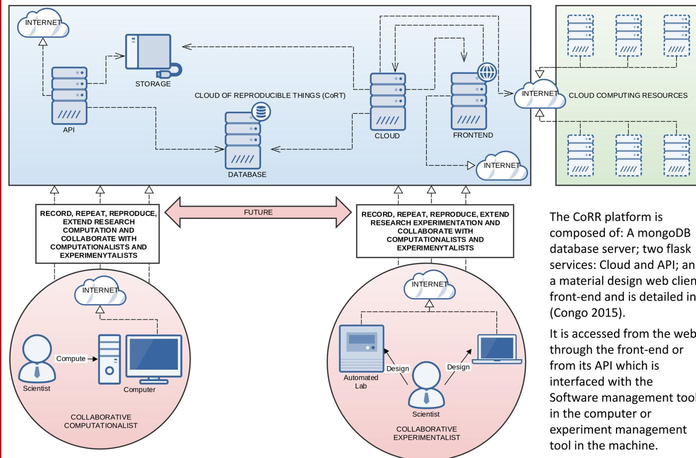
The CoRR platform is composed of: A mongoDB database server; two flask services: Cloud and API; and a material design web client front-end and is detailed in (Congo 2015).
