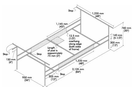
Figure 6. Steel Test Frame for Dead Weight Stiffness Test
