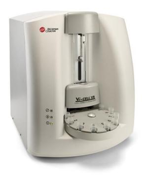
Fully automated, computer-operated image analyzer that uses the Trypan Blue Dye Exclusion Method for Viability, Cell Counting and Total Cell Concentration.
