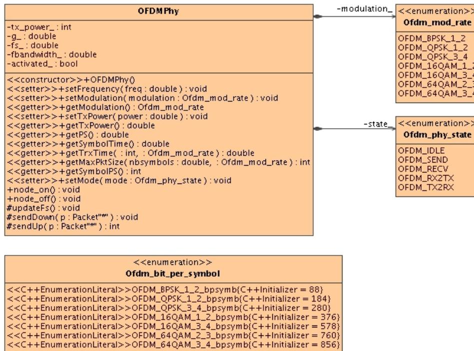
**Figure 17: OFDM Physical layer class diagram**
