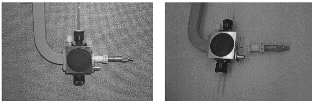
Fig. 2. Adjacent reference sample device manufactured by Bruker Instruments. Left: Assembled cavity with the reference sample device attached and quartz holder for alanine pellets. Right: The same construction in the disassembled form; the dark ruby rod and the illumination grid used for its insertion can be seen.
