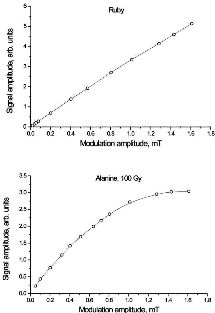
Fig. 7. Dependence of the amplitudes of ruby and alanine signals on modulation amplitude. Least-squares fit for the alanine dependence in the range 0.05–0.8 mT:  $Y = 0.474 + 3.877x - 1.252x^2 + 0.000413x/\ln x$ ; standard error of the fit is 0.012.
